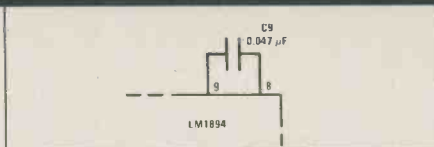
Fig. 2. If the multiplex filter is omitted, connect C9 across pins 8 and 9 as shown. Illustrations are courtesy of National Semiconductor.
