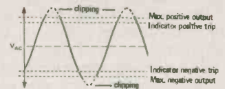
Fig. 1 Illustrating clipping of a sine wave by output overload.
