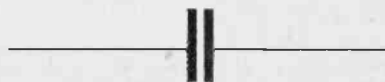
Fig.2. Symbol for capacitor. This symbol is used for a fixed capacitor, meaning a capacitor whose value is not deliberately changed (as for tuning a radio). A slightly different symbol is used for an electrolytic capacitor.
