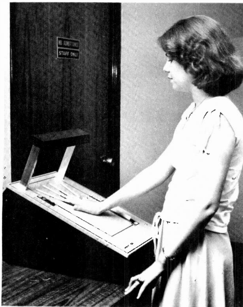
With Identimat, the operator places the complete palm on the glass, the system then checks various dimensions and the 'print' to ensure complete security.
