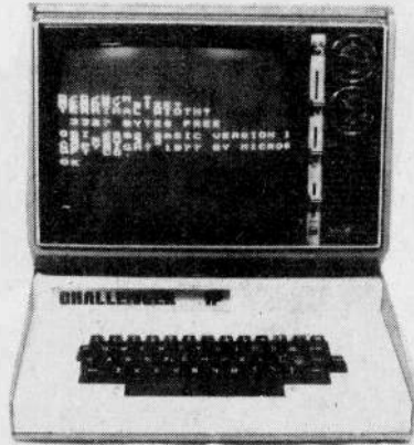
Fig. 1. Challenger 1P, with converted TV used for display
