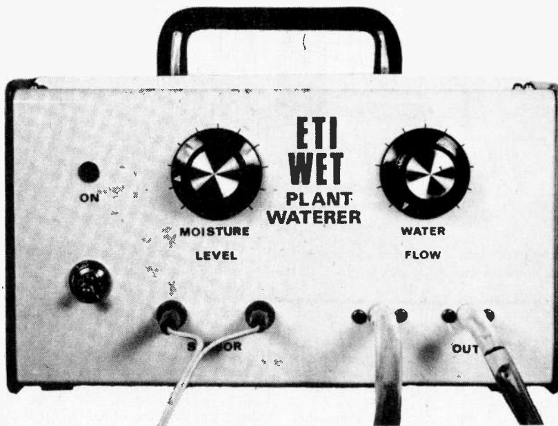
Head on view of the completed prototype, the LED can be left out if you want extended battery life.
