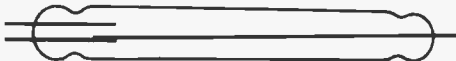
Fig. 15. This type of reed switch may be used for either change-over or normally closed operation.
