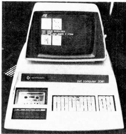
This futuristic looking unit is the much talked about PET from Commodore — note the unusual keyboard layout.
