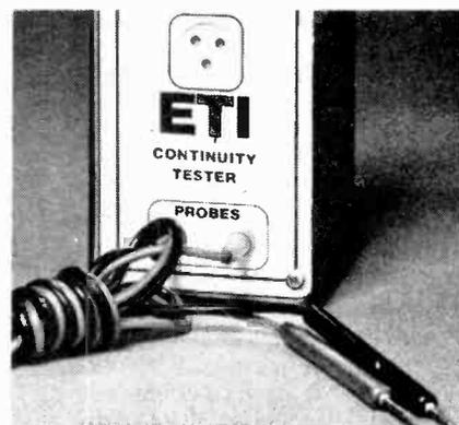
NOT your hackneyed multivib with a break in the supply rail but a properly designed unit which will tell you if there's continuity and very little else — no voltages to turn on transistors etc.
