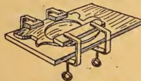
Cramp the wood down when gluing parts together.
