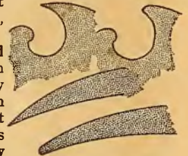
Good and bad cutting in common designs.
