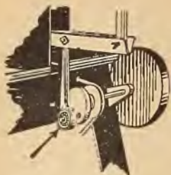
The ball bearing Pitman in position on the machine.
