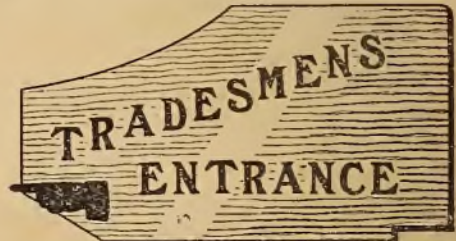
The lettering is cut in wood and glued on a backboard, before being painted or stained. The index is a distinctive feature.
