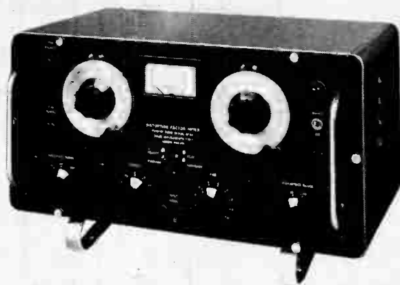
Fig. 6. Distortion Factor Meter for total wave distortion
