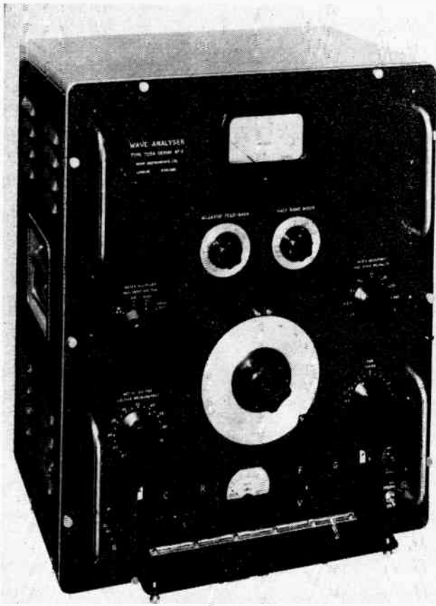
Fig. 3. Wave Analyzer gives accurate harmonic measure
