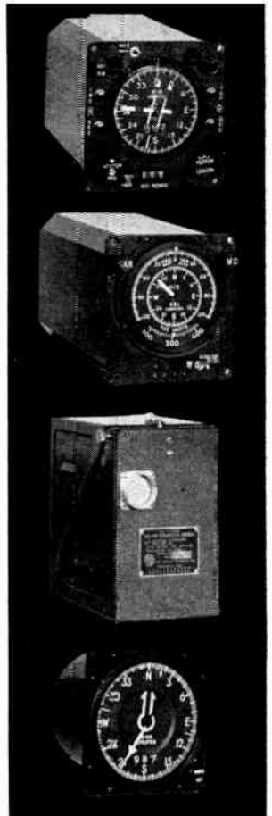
Three basic units of the R-Theta Computer System and the repeater (bottom)
