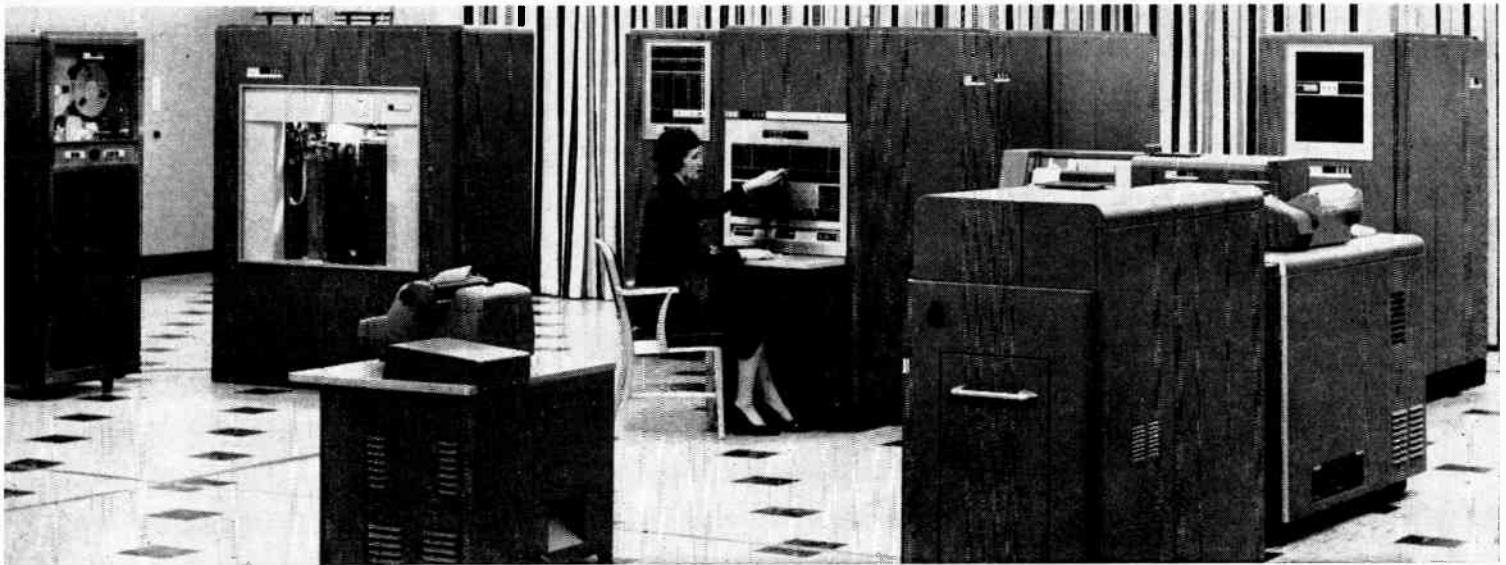
Digital data-processing system including magnetic tape handling units, random access memory and main computer console
