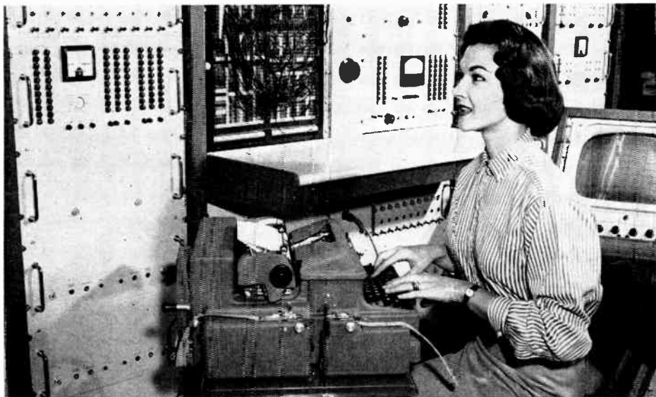
Operator types program for analog computer on machine which punches paper tape
