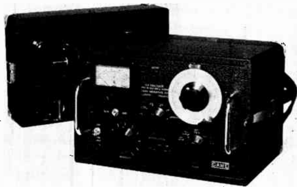
Fig. 2. A.F. Analyzer for general sound and vibration work
