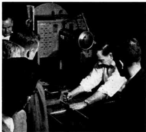
Punching out printed circuit boards on the Wales Hydra New-Matic looked fascinating to the IRE visitors.
