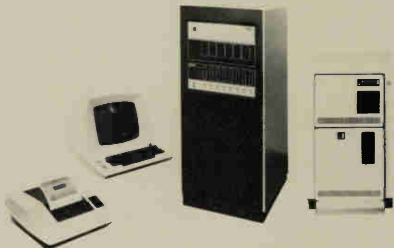
Components of a typical voice response order entry system are shown in this system from Interface Technology Inc. From left: logging printer, CRT display, Touch-Tone/Voice response subsystem, and the IBM Series/1 computer.
