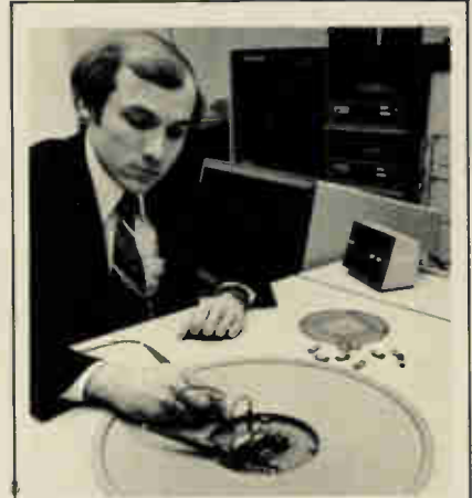
Production testing of complex large scale integrated circuits gets a boost with chip tester developed at Bell-Northern Research. Unit performs 1.5 million measurements in 45 seconds, approaching the limits of the laws of physics. New system is more accurate than any other in existence and is used at the Northern Telecom semiconductor manufacturing plant in Ottawa.
