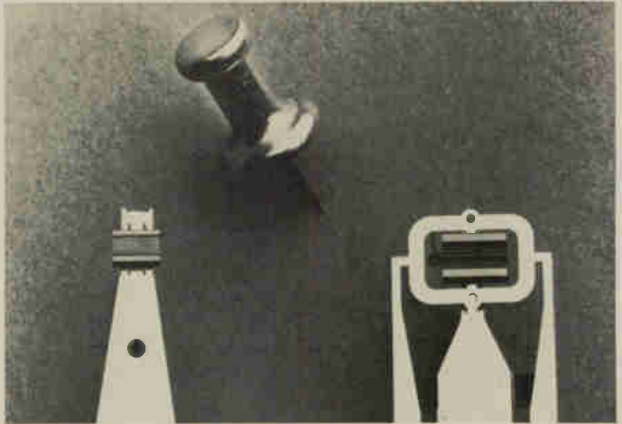
New thin film read/write head (left) in Seagate ST512 5¼-in. micro-Winchester drive compared with standard ferrite type head. Thin film head can read data with higher packing densities on the total surface of the disc, allowing more data to be compressed into same disc space.
