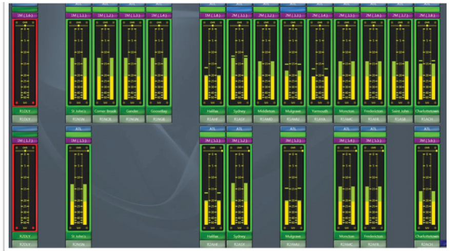
Figure 3 (above) shows the presentation display while an alert message is being inserted on the Sydney and Mulgrave Radio One feeds, as indicated by the blue bars above the audio meters.
