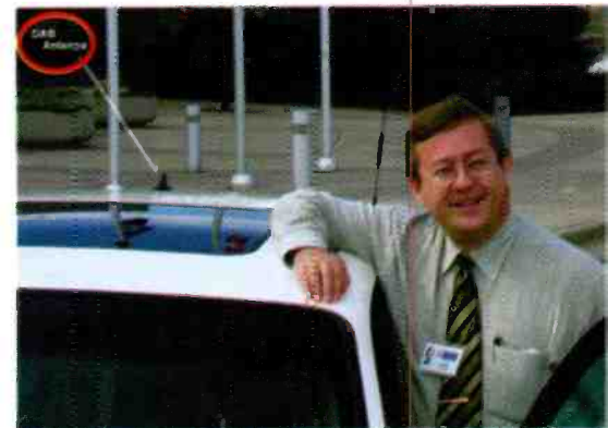
John Wood, GM's manager, R&D and Technology, beside the Impala outfitted with a fully-functional DAB receiver. The small black 'shark fin' mounted at the back of the roof-line is the DAB antenna.
