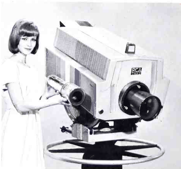
This is the 4-1/2 inch image orthicon tube used in the luminance channel to sharpen the picture.
