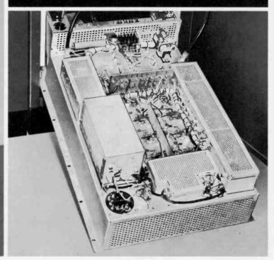
Aural and visual exciter circuits mounted on a single hinged chassis
