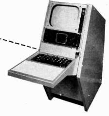
Preset controls on the Camera Control Panel are under a hinged cover - here shown open. A 14" picture and 5" waveform display are provided by the BD 873 Monitor.
