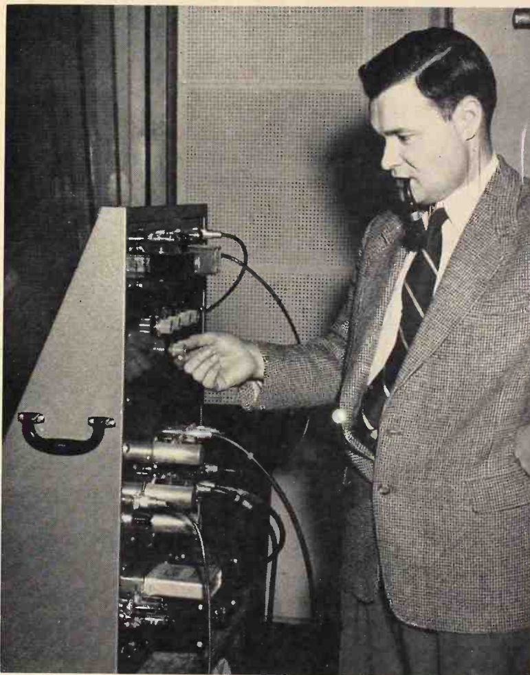
DIRECTOR OF ENGINEERING Bill Jeynes, of CHCH-TV, Hamilton demonstrates his new special effects generator. The new instrument is portable, has one-quarter the parts of existing models, costs one-seventh the price, is more flexible technically and can be operated by anyone, experienced or not. In the device, Bill has perfected the circular iris effect, and has equipped his own station with it, making CHCH-TV the only station capable of producing circular segmentation.
