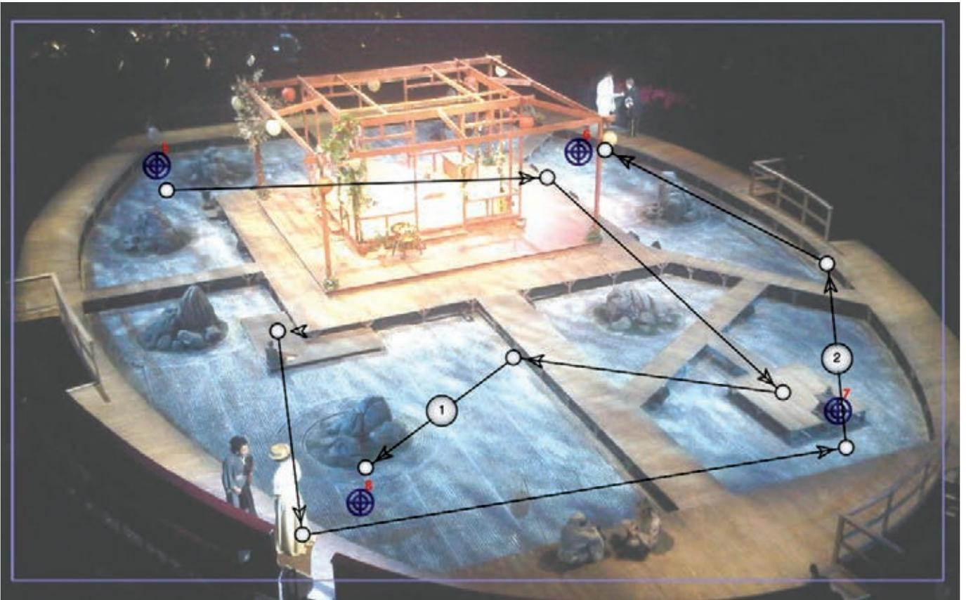
TiMax PanSpace graphical user interface permits localization of performers and sound effects by dragging objects around a jpeg of the stage or field or play.
