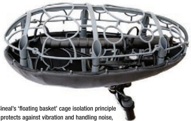
Cineal's 'floating basket' cage isolation principle protects against vibration and handling noise, using four flexible 'U' isolators in its mic windshields.
