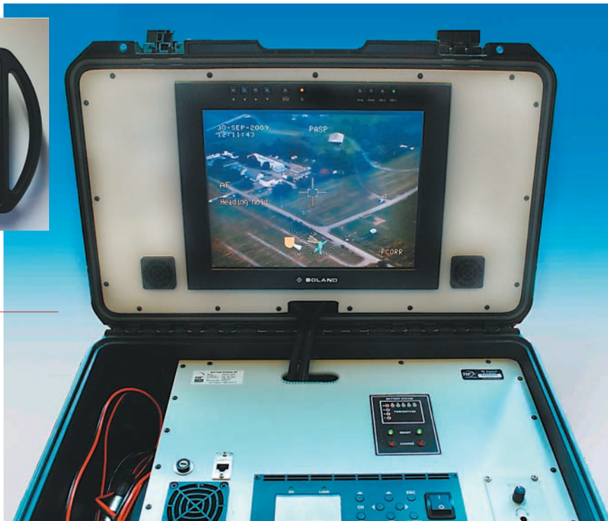
New COFDM systems from RF Extreme can receive up to six microwave feeds in non-line-of-sight production applications.
