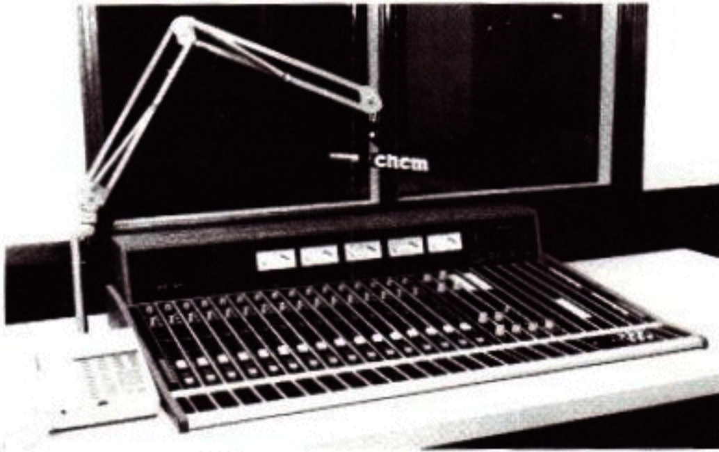
Production Control Room. McCurdy 16-channel board mixes the inputs from 2 McCurdy turntables, 2 PR-99 Revox tape machines, 2 Fidelipac CTR-14 cart machines, Technics cassette machine, local mic, 2 announce booths, satellite and microwave feeds. The entire audio system within the station is stereo, in anticipation of AM stereo operation. In the meantime this provides a degree of equipment redundancy, which engineering appreciates!
