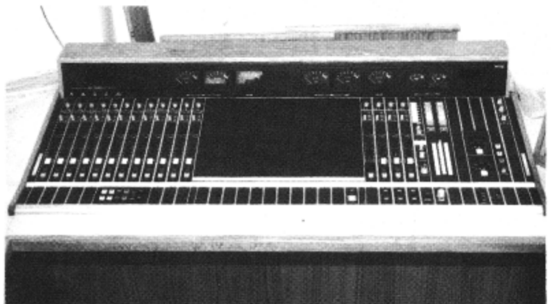
Custom-designed consoles were supplied by McCurdy, pre-wired and fully tested. Large script board is provided in centre, mic and other functions used constantly are at right, with peripheral equipment at left.
