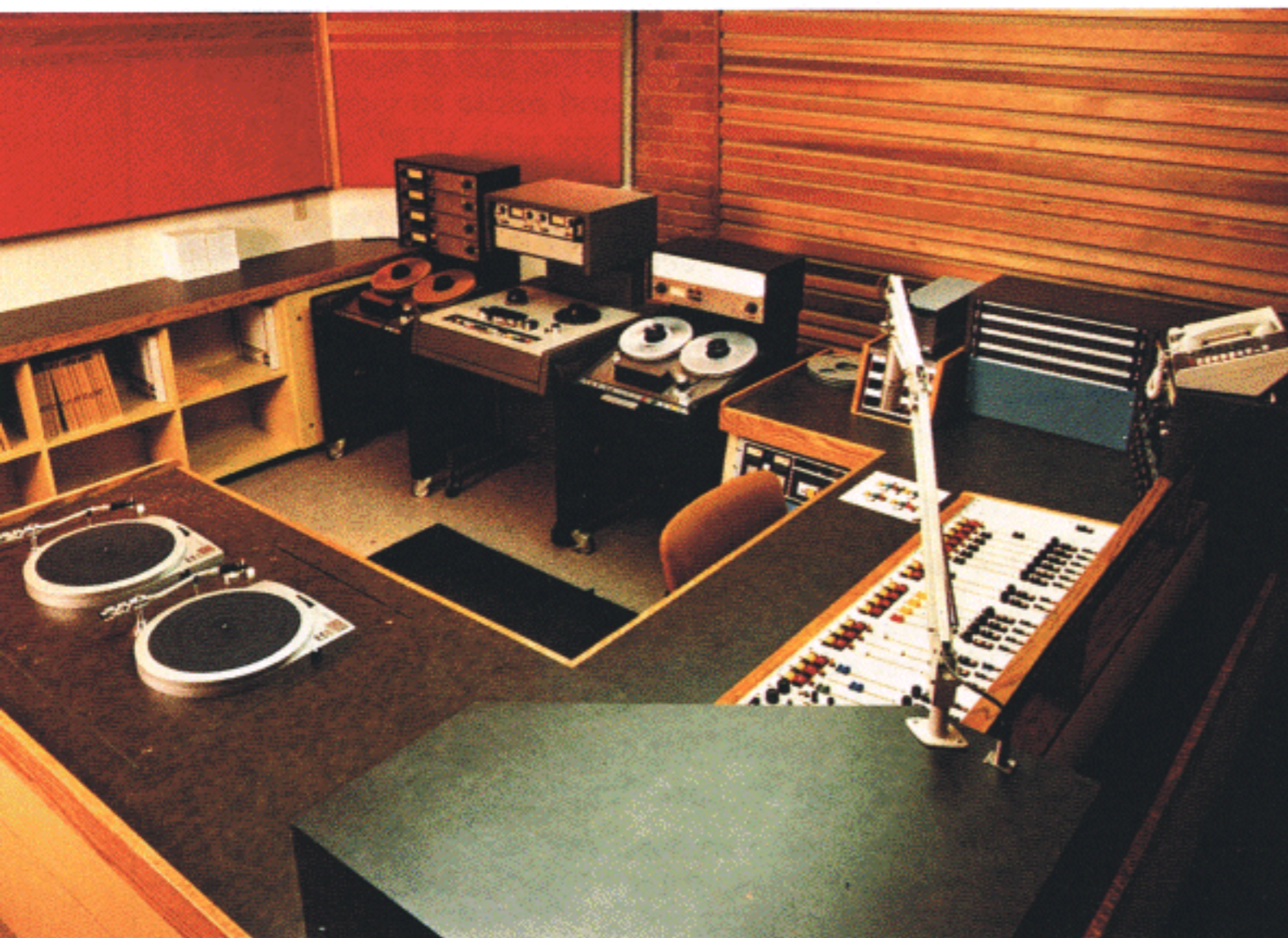
Production control room is complete with 4-track, 2-track and full track recording. The equipment turrets contain patchfields, graphic equalizers, reverb, flanger and input selector units. Reel-to-reel remotes are at operator's left. Turntables are flush-mounted on neoprene isolators and a cavity under the turntable is filled with 60 kgs. of sand.
