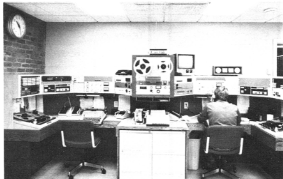
Newsroom is equipped with six work stations, two of which are shown here. The cockpit design of each position places more equipment within easy reach of news announcer. James Losh is working at position 2.
