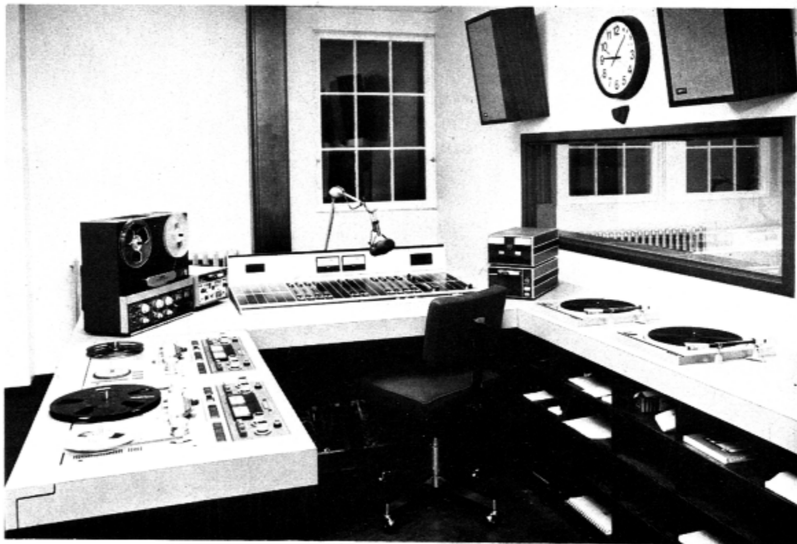
Production control room includes Ward-Beck board, three Studer Revox tape machines (two B67s, one B77), two Technics turntables, Ampro and ITC cart machines and Advent speakers. Equipment was supplied by Caldwell and installed by CJMX-FM technical director Henry Albert, assisted by Alan Aysto. (Photos by Tramontin Photography, Sudbury.)
