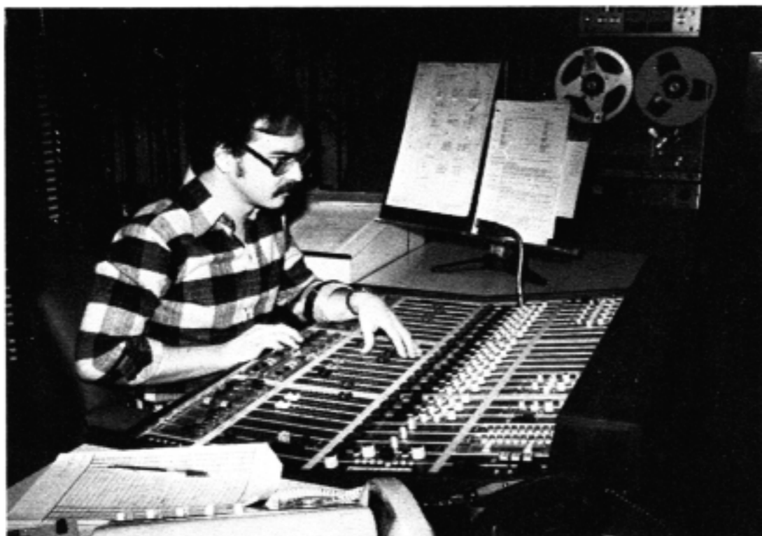
On-air AM master control room is equipped with new McCurdy SS8600 console. Bob Pinkney is at controls. Room is equipped with PSB Beta speakers, made in Canada. Tape seen in background is daily logging machine.
