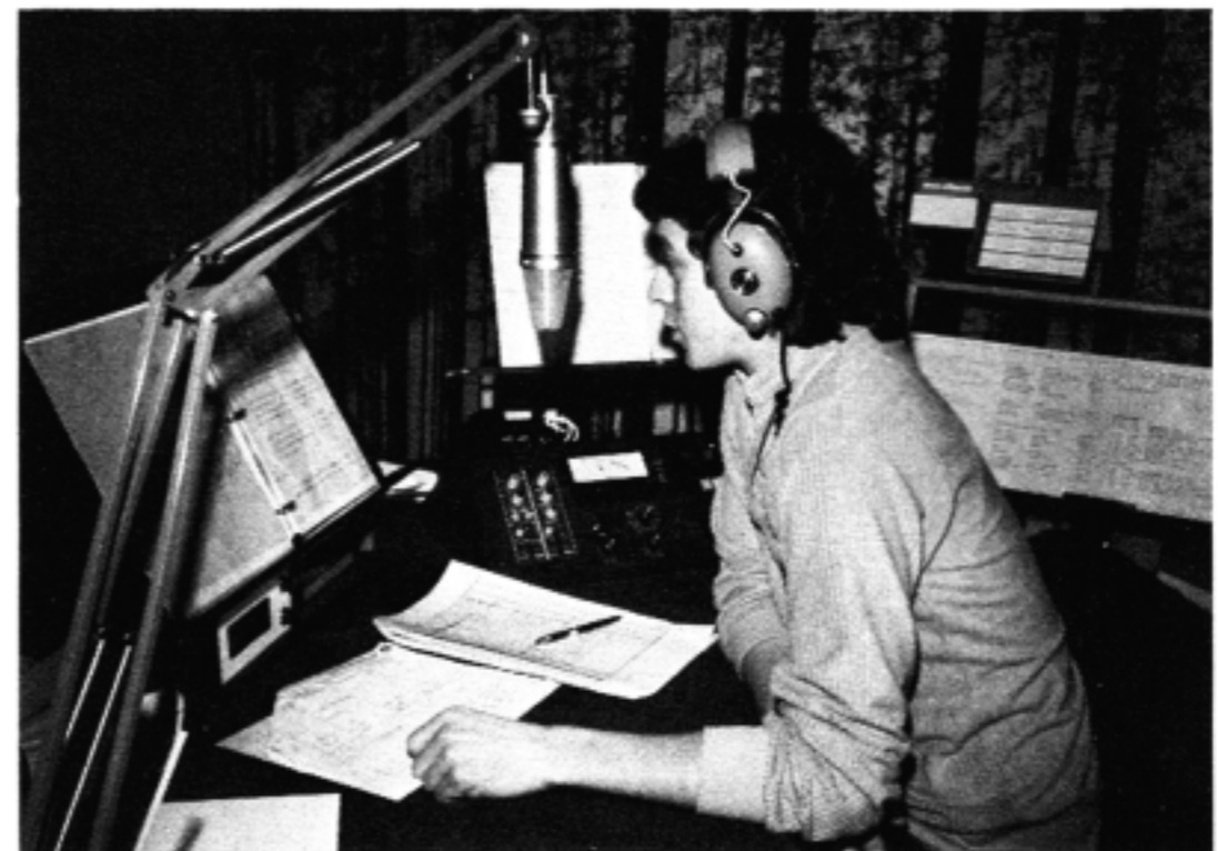
Announcer John Majhor at work in studio, equipped with turret controls for monitoring either off-air or direct. Note digital thermometer and clock. Microphone is Neumann U-87, speaker is PSB Avantié.
