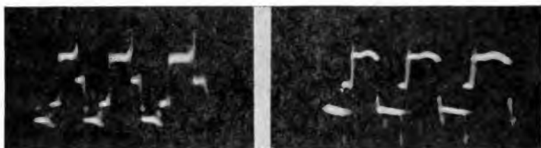
Figs. 378, left, 379, right. The waveform taken in the primary circuit when the buffer condenser was removed is shown in Fig. 378. The waveform of the secondary circuit under similar conditions is shown in Fig. 379.
