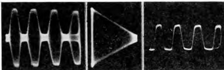
Fig. 428 (left) shows the modulated wave envelope when the modulator is matched to a 2000-ohm load. The corresponding trapezoidal pattern is shown in Fig. 429 (middle) and the audio voltage across the modulator load is shown in Fig. 430 (right). Compare these images with Figs. 393 and 394.
