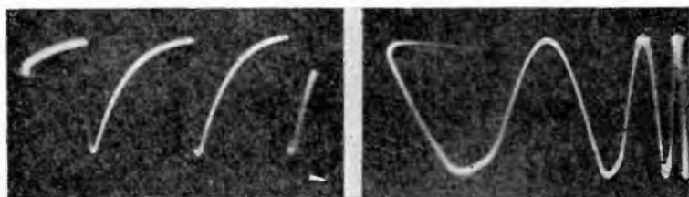
Fig. 89, left, Fig. 90, right. The same wave as shown in Fig. 88-A is shown in Fig. 90 when spread across the screen with a non-linear sweep, as illustrated in Fig. 89. Note how the right side of the image is crowded due to the non-linearity of the sweep.
