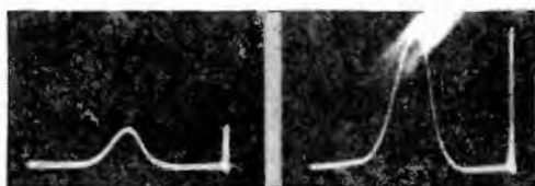
Figs. 326, left, 327, right. The low amplitude of the curve of Fig. 326 makes interpretation of its characteristics difficult. Note the difference in Fig. 327, in which the amplitude is correct.
