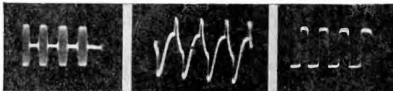
Fig. 230-A, left, Fig. 230-B, middle, Fig. 230-C, right. A. The wave envelope of the modulated output of a commercial test oscillator. B. The a-f. output of the same oscillator. C. The a-f. signal resulting from demodulation of the modulated wave shown in A.
