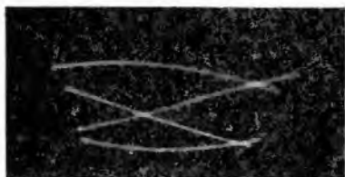
Fig. 78. By applying too much synchronization to the pattern of Fig. 77, the image at the left was obtained. Note that the pattern is no longer symmetrical.
