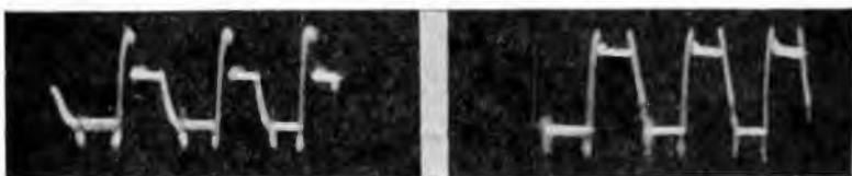
Figs. 376, left, 377, right. The oscillogram of Fig. 376 was made after the contacts had been restored to normal. When a .5-ohm resistor was connected in series with the battery, the oscillogram of Fig. 377 was obtained.
