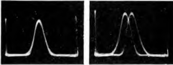
The left pattern shows the circuit in resonance and that at the right, the circuit out of resonance. These oscillograms made with the Supreme 555.
