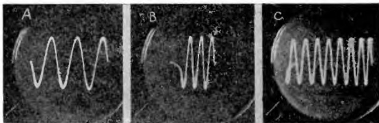
Fig. 68. The sweep amplitude of A is the same as that in Fig. 67-C, but the sweep frequency has been reduced so that three cycles appear on the screen. When the amplitude of the sweep is reduced, as in B, the peaks of the waves become sharp and make it difficult to get a true idea of the wave's shape. In C the sweep frequency has been further reduced with the result that the peaks are more pointed than in B.
