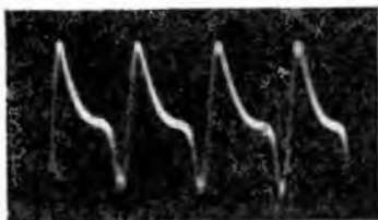
Fig. 233. The a-f. output of a commercial test oscillator. This oscillator is also responsible for the modulated patterns shown in figures 234 to 236 inclusive.
