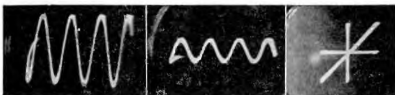
Figs. 207, left, 208, middle, 209, right. The output wave of the Class A stage is shown in Fig. 207. The input voltage wave to the Class B stage is shown in Fig. 208. The correct phase relation of 180^\circ between the two voltages to the Class B input is indicated in Fig. 209.
