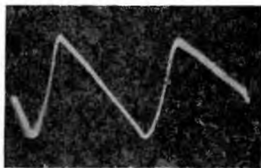
Fig. 41. The sweep of the Egert oscillograph is different from those shown before. Here the charging portion of the cycle is steep and the discharge is more gradual, both parts of the cycle being used for sweeping the spot across the screen. Compare this wave with that of Fig. 35.
