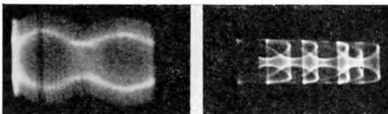
Fig. 431 (left) is an example of hum modulation of the carrier, which is modulated at 1000 cycles. Fig. 432 (right) is an example of a pattern resulting from incorrect test connections.
