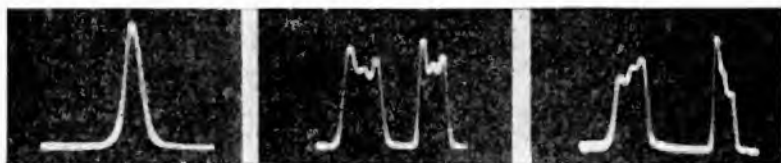
Figs. 268, left, 269, middle, 270, right. The sweep frequency used in developing the symmetrical pattern of Fig. 268 was twice the motor frequency. Compare with Fig. 265. Figs. 269 and 270 are examples of asymmetrical resonance curves. Explanation of the dissimilarity of the curves is given in the accompanying text.
