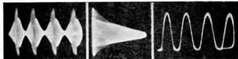
Fig. 418 shows the modulated wave. Fig. 419 shows the corresponding trapezoidal pattern and Fig. 420 shows the audio wave across the modulator output during the operative condition stated. The sudden start and cessation of the uncontrolled oscillation is clearly shown in Fig. 418.
