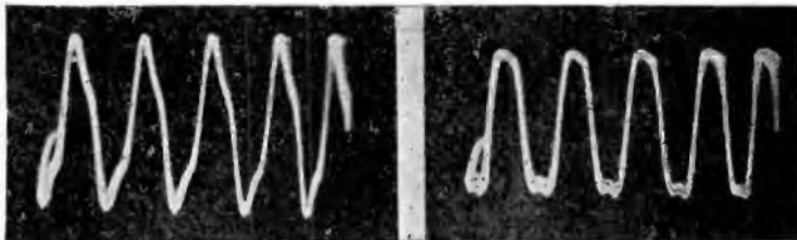
Figs. 165, left, 166, right. The composite wave of the waves shown in Figs. 163 and 164. Note the effect on the shape of the composite wave that a shift in phase has. See Fig. 166.
