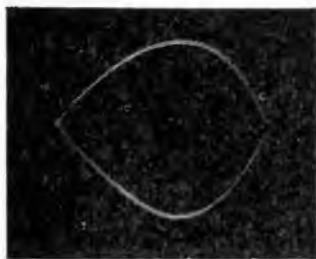
Fig. 73. The image resulting when the sweep frequency is twice the frequency of the wave being observed. Compare Fig. 27. Such a pattern is difficult to stop on the screen, as the points are moving on the fastest portion of the cycle. The top and bottom halves of the wave should coincide.
