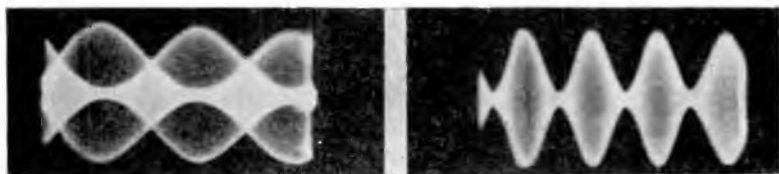
Figs. 387, left, 388, right. When the sweep voltage is incorrectly adjusted a pattern like that of Fig. 387 results. A correctly adjusted sweep voltage yielded the oscillogram of Fig. 388.
