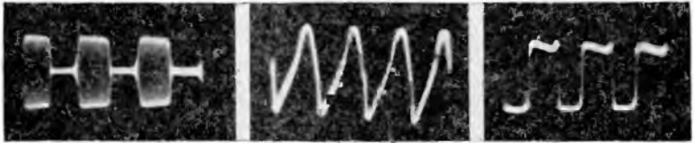
Fig. 231-A, left, Fig. 231-B, middle, Fig. 231-C, right. A. The wave envelope of the modulated output of a commercial oscillator. B. the a-f. output of the same oscillator. C. The a-f. signal resulting from demodulation of the modulated wave shown in A.
