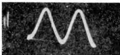
Fig. 136. The waveform of the voltage produced by magnetic deflection applied vertically. The frequency of the wave is the same as in Fig. 135, the horizontal sweep frequency having been changed to get two cycles on the screen.
