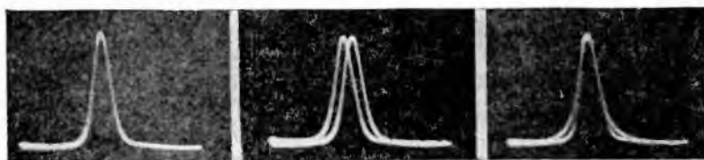
Figs. 299, left, 300, middle, 301, right. These resonance curves show correct alignment of a symmetrical circuit as to frequency and band width (Fig. 299), alignment at the wrong frequency, (Fig. 300), and alignment at the correct peak but improper response over the band, (Fig. 301).
