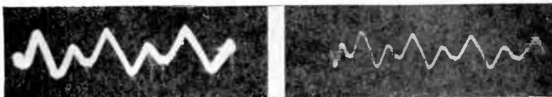
Figs. 372, left, 373, right. Oscillogram of voltage taken across V and V1 is shown in Fig. 372. Fig. 373 shows the voltage across the same points, but with a shorter exposure of the photographic film. Note the transients in Fig. 372, indicated by the faint vertical lines below the wave, but not visible in Fig. 373.
