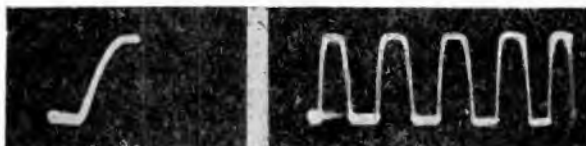
Figs. 185, left, 186, right. A further increase of input to the amplifier developed the characteristic of Fig. 185. That the positive swing was excessive was proved by the output waveform of Fig. 186.
