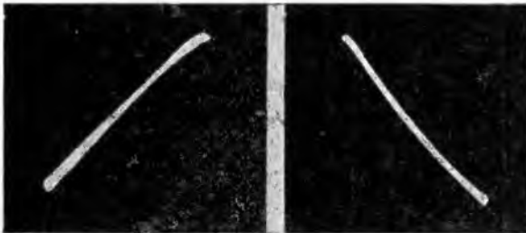
Fig. 95. A, left, B, right. Both patterns show a 1-1 ratio between the frequencies. The phase difference in A is 180^\circ and that in B is 0^\circ .
