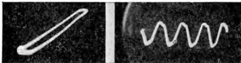
Figs. 191, left, 192, right. When the volume control was further advanced the ends of the voltage characteristic became slightly flattened, see Fig. 191, and a change from a sine wave is evident in the output wave, see Fig. 192.
