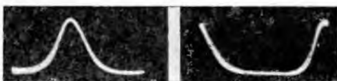
Figs. 316, left, 317, right. Curves showing correct and incorrect polarity of impulse generator signal appear at left and right.
