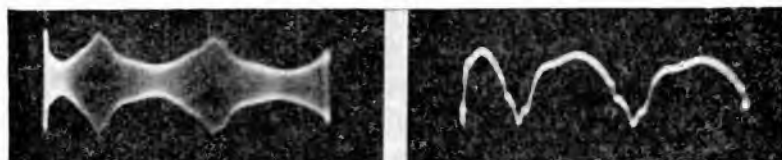
Fig. 236-C, left, Fig. 236-D. The modulated output waveform of the same oscillator when adjusted to 1700 kc., is shown in C. The a-f. output resulting from the demodulation of C is shown in D.
