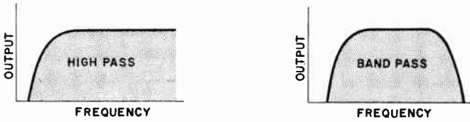
Fig. 13-6. Horn is changed from high-pass element to band-pass element by allowing throat cancellation to take place. This is permissible where horn is applied to woofer. Horn thus acts as high end rolloff for woofer section.
