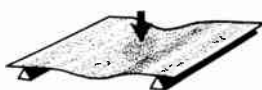
A FLAT PIECE OF PAPER SUPPORTED AT ITS EDGES WILL READILY SAG AND DISTORT UNDER PRESSURE APPLIED TO ITS CENTER
