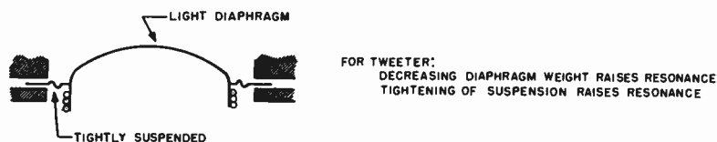
Fig. 3-11. To achieve high natural resonance, tweeters have small, light diaphragms, stiffly supported.
