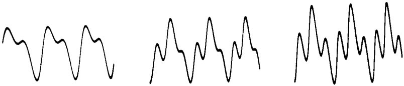
Fig. 3-3 Complex waves made up of several sine waves of different frequencies.
