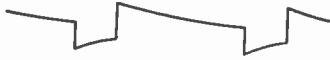
FIG.4-18. Typical wave form of condenser current or suppressor voltage for the circuit of Fig. 4-17.
