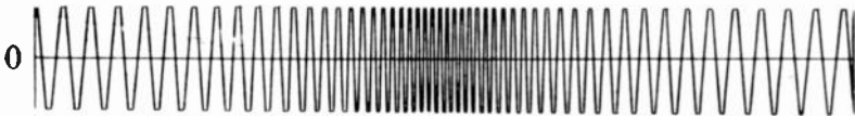
FIG. 6-9. Current i = dq/dt in eq. (6-28); \omega_o / \omega_s = 40 ; k as indicated. amplitude, and one of the advantages of frequency modulation is that amplitude modulation can be clipped off the wave without substantial harm to the frequency modulation.
