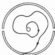
FIG. 10-22. Motion of an electron that delivers energy to a source of alternating potential between magnetron plate segments.
