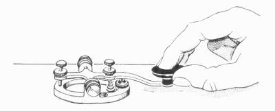
THE CORRECT METHOD OF HOLDING THE KEY WHEN TRANSMITTING
