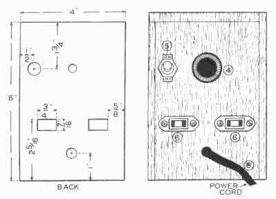
DETAILS OF THE BACK OF THE CABINET SHOWING OPENINGS FOR RESET SWITCH, CONTROL, SOCKETS, AND POWER CORD
