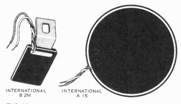
TWO OF THE SELENIUM CELLS USED TO BUILD APPARATUS DESCRIBED IN THIS BOOK
