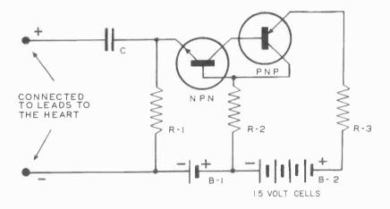
The circuit of the cardiac pacemaker, showing conventional schematic symbols that represent two transistors, three resistors, a capacitor, and five small mercury batteries.
