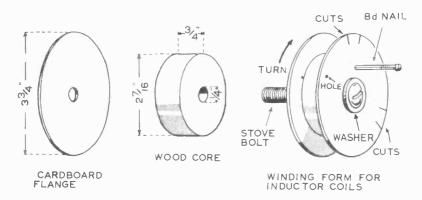
THE FORM FOR WINDING THE COILS
