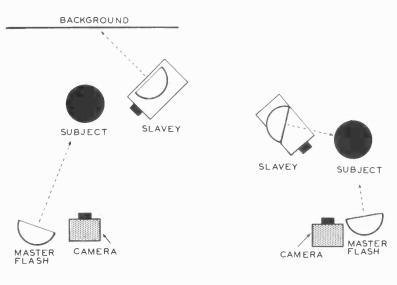
DIAGRAMS SHOWING HOW THE SLAVEY IS POSITIONED TO AID IN LIGHTING Direct light from slavey should not shine into camera.
