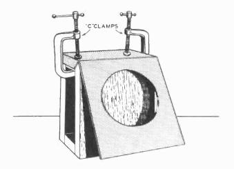
THE TOP AND FRONT OF THE METAL CABINET The top and front of the form and two "C" clamps are used to bend the metal in this operation.
