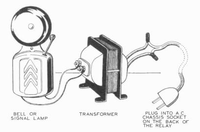
An electric bell can be used as the signal device by connecting it to a bell-ringing transformer.
