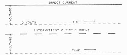
AN ENGINEER'S PICTURE OF DIRECT CURRENT
