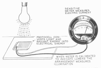
THE PRINCIPLE OF THE LIGHT METER AND EXPOSURE METERS USED TO MEASURE ILLUMINATION
