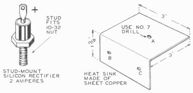
A STUD-MOUNT SILICON RECTIFIER MUST BE KEPT COOL BY A HEAT SINK
