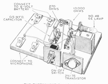
THE PHOTOPHONE TRANSMITTER The letters E, B, and C identify the wires connected respectively to the EMITTER, BASE, and COLLECTOR of the transistor.
