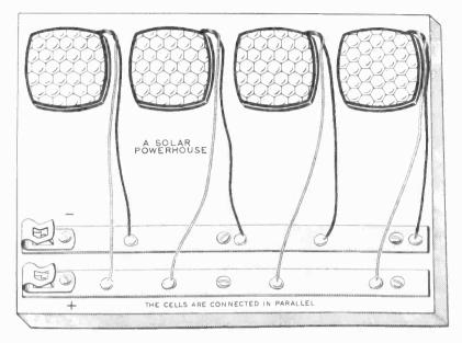
FOUR SIM SILICON CELLS CONNECTED IN PARALLEL
