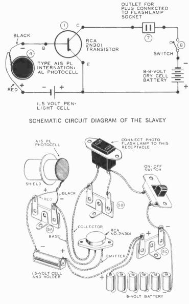
PICTORIAL WIRING DIAGRAM OF THE SLAVEY
