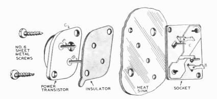
MOUNTING KIT FOR A POWER TRANSISTOR
