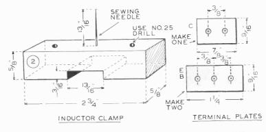
DETAILS OF INDUCTOR COIL CLAMP, ROTOR PIVOT, AND TERMINAL PLATES
