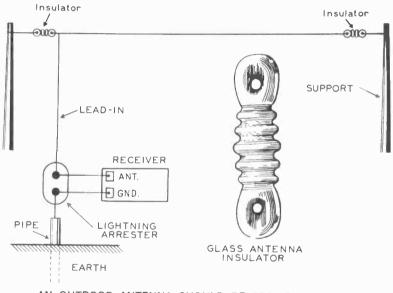
AN OUTDOOR ANTENNA SHOULD BE PROVIDED WITH A LIGHTNING ARRESTOR
