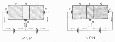
The arrangement of the semiconductor materials in the PNP and NPN junction transistors.
