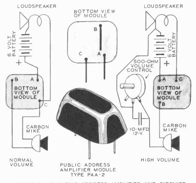
MODULE PAA-2 PUBLIC ADDRESS AMPLIFIER AND CIRCUITS When the amplifier is used in a room of average size, make the circuit connections as shown in the left-hand diagram. If more volume is required for a large room or small hall, use the hookup shown in the right-hand circuit diagram.
