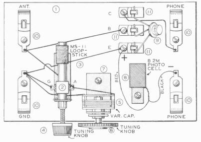
PLAN OF RADIO RECEIVER WITH DIODE DETECTOR AND TRANSISTOR AMPLIFIER
