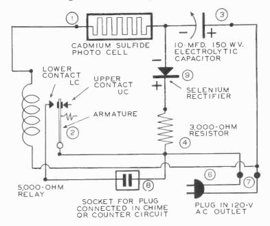
SCHEMATIC CIRCUIT DIAGRAM OF THE AUTOMATIC LIGHT SWITCH ARRANGED TO LIGHT A LAMP, RING A CHIME, OR OPERATE A COUNTING DEVICE
