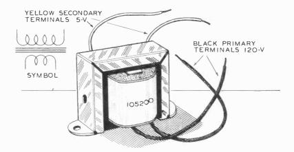
NO. 105200 STEP-DOWN TRANSFORMER, 120-V PRIMARY, 5-VOLT SECONDARY
