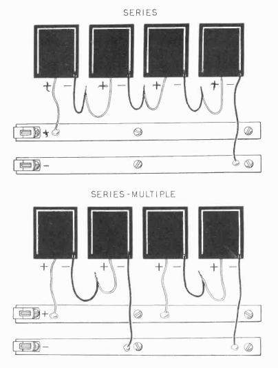
SERIES AND SERIES-MULTIPLE CONNECTIONS FOR FOUR CELLS
