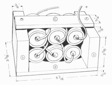
THE 9-VOLT BATTERY AND BATTERY HOLDER How to connect six flashlight cells in series to form a 9-volt battery.
