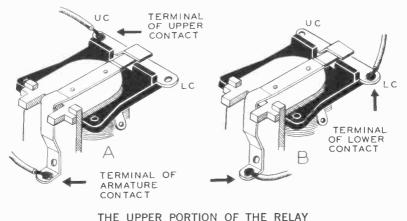
The letters UC and LC are abbreviations for "upper contact" and "lower contact."
