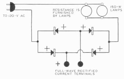
SCHEMATIC CIRCUIT DIAGRAM FOR FULL-WAVE RECTIFIER
