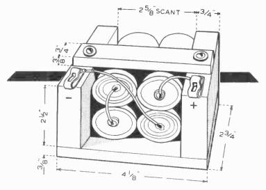
BATTERY HOLDER FOR FOUR SIZE-D CELLS
