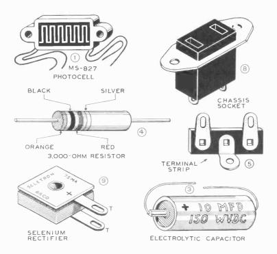
THE PRINCIPAL COMPONENTS USED IN BUILDING THE LIGHT SWITCH The terminals of the rectifier are marked T in the illustration. The positive terminal is identified by a plus sign.
