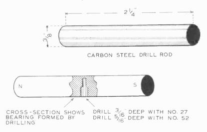
DETAILS OF MAGNETIZED ROTOR MADE OF DRILL ROD
