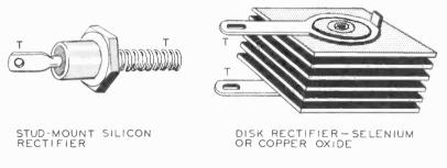
SMALL SEMICONDUCTOR RECTIFIER UNITS The letter T indicates the rectifier terminals.
