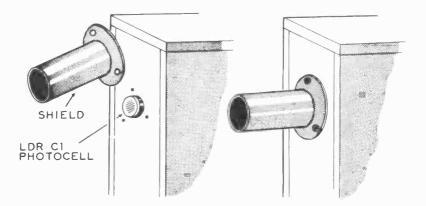
The shield is fastened to the front of the cabinet and protects the cadmium sulfide photocell from all light except that which enters the front end of tube.
