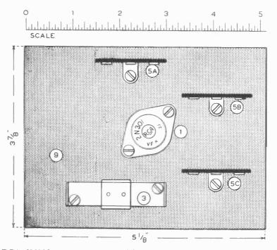
RCA 2N301 power transistor (1). 1.5-volt AA dry cell holder (3). Tiepoints (5A), (5B), and (5C).
