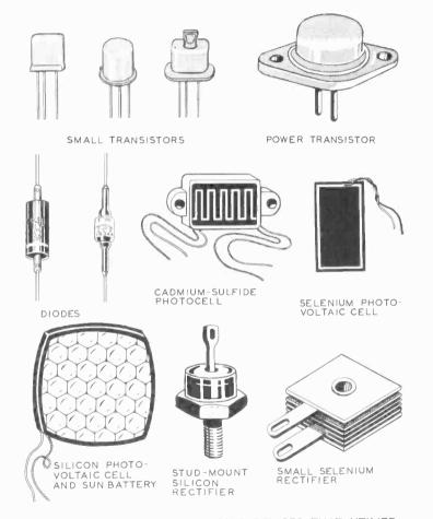
SOME WIDELY USED ELECTRONIC DEVICES THAT UTILIZE SEMICONDUCTOR MATERIALS IN THEIR CONSTRUCTION (Consult the glossary and index for descriptions and explanations of these components of electronic circuits.)
