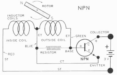
SCHEMATIC CIRCUIT WHEN AN NPN TRANSISTOR IS USED Notice that the polarity of the battery is reversed so that the collector (C) is positive. One terminal (ST) of the inside coil is connected to the negative terminal of the battery. The other terminal (CT) of the inside coil is connected to the emitter.
