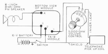
CIRCUIT FOR CONNECTING TELEPHONE AMPLIFIER MODULE, LOUDSPEAKER, VOLUME CONTROL, AND TELEPHONE PICKUP COIL FOR GROUP LISTENING
