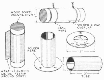
THE SHIELD This consists of a tube and flange made of thin sheet metal.
