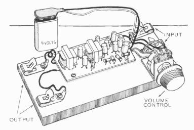
SUBMINIATURE 4-TRANSISTOR AMPLIFIER MOUNTED ON WOOD BASE WITH VOLUME CONTROL AND TERMINAL CLIPS This is the same amplifier shown in the preceeding illustrations, but the components have been assembled on the printed circuit board in a reversed position.
