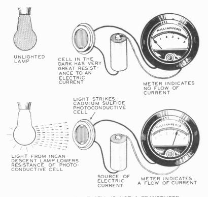
A PHOTOCONDUCTIVE CELL IS NOT A TRANSDUCER It does not convert light into an electric current. Light causes it to vary its ability to CONDUCT an electric current. A photoconductive cell in the dark has very great resistance to the flow of electric current. Exposure to light lowers this resistance.
