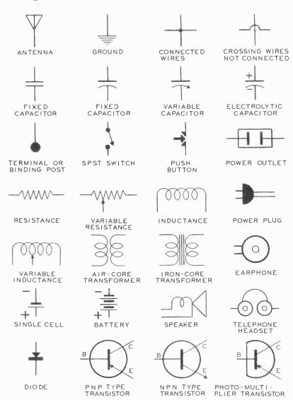
SYMBOLS USED IN DIAGRAMS OF SCHEMATIC RADIO CIRCUITS Here and in the illustration that follows are the symbols used in the schematic circuit diagrams in this book.
