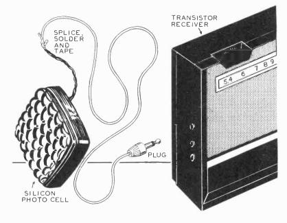
THE AUDIO AMPLIFIER IN A PORTABLE RADIO RECEIVER MAY BE UTILIZED AS PART OF THE PHOTOPHONE BY CONNECTING IT TO A SILICON PHOTOCELL (Consult Chapter 12 for additional suggestions.)
