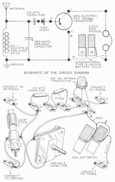
PICTORIAL CIRCUIT OF DIAGRAM OF RECEIVER
