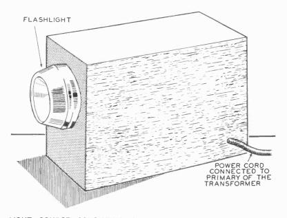
LIGHT SOURCE CONSISTING OF WOOD CABINET ENCLOSING A FLASHLIGHT WITH 6.3-VOLT LAMP OPERATED ON A FILAMENT TRANSFORMER
