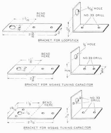
BRACKETS FOR MOUNTING THE LOOPSTICK AND TUNING CAPACITOR When these parts are not furnished with the components, they can be made out of sheet metal.
