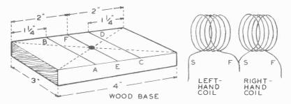
THE WOOD BASE FOR THE GALVANOSCOPE The text explains how to locate the guide lines and coils.
