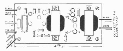
1-WATT, 4-TRANSISTOR, PUSH-PULL AUDIO AMPLIFIER T1, T2, T3, and T4 are transistors. HS indicates radiating fins to dissipate heat.
