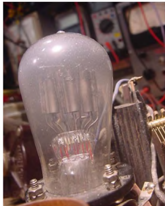
The 'Emerson Multivalve' (triple triode, circa. 1926)
