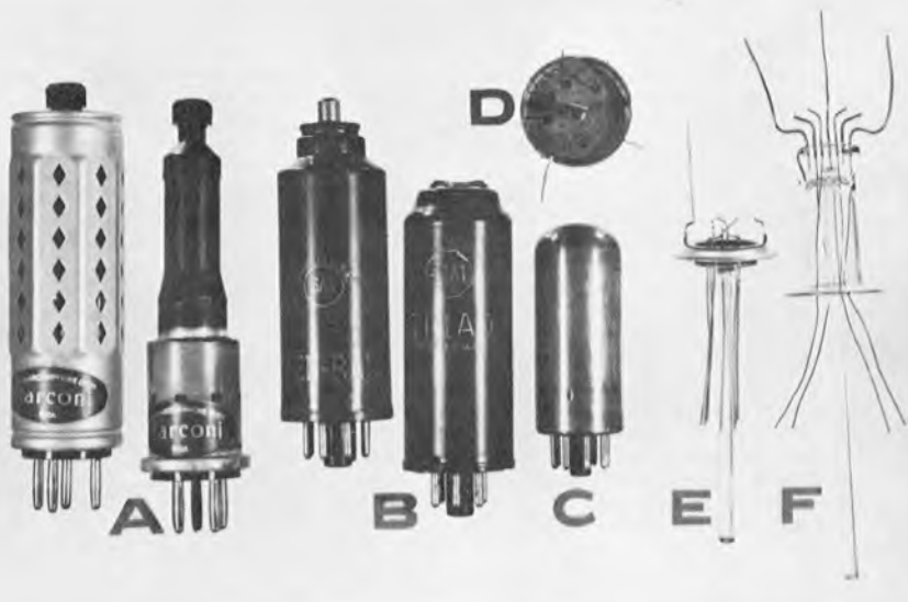
(A) Catkin tubes (B) MG tubes (C) Bullet (D) Early metal tube header (E) Glass button stem header (F) Old style press seal.
