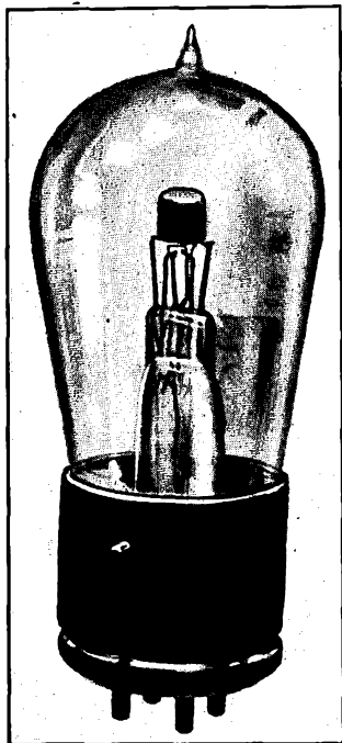
FIG. 130.—General Electric type Receiving Tube. Length: 10 cms.
