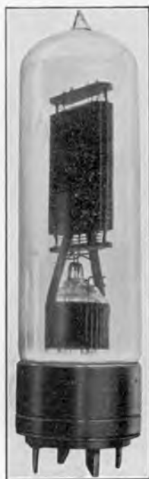
FIG. 137.—Western Electric Type Power Tube. Length: 30 cms.
