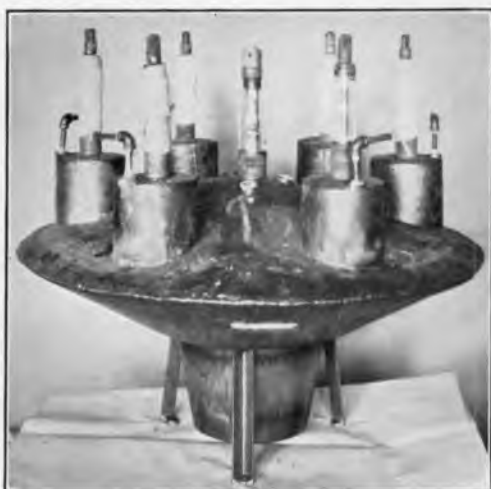
FIGURE 20.—Small iron-tank rectifier with no clamped joints.
