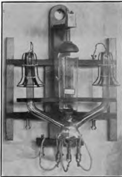
FIGURE 28.—Series arc tube in tube holder and fitted with static protectors.
