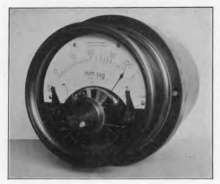
FIG. 128. Brown Boveri contact-making vacuum meter.
