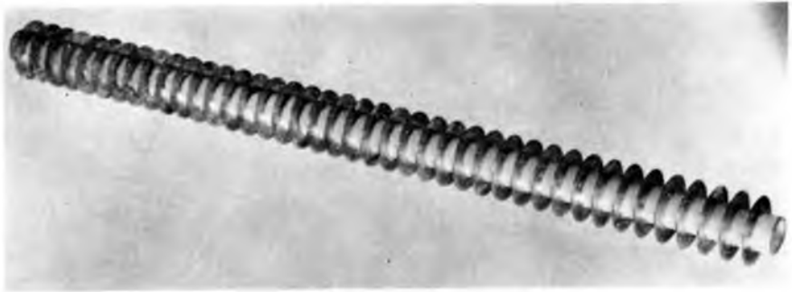
Figure 14.5. Stacked assembly of 41 copper disks sealed to intermediate ceramic rings with SEL mix No. 101. (Courtesy Stanford Electron Devices Laboratory.)
