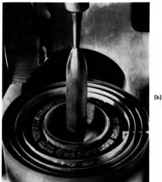
Figure 4.18. Improved Czochralski crystal pulling furnace; a) graphite heater; b) crystal, crucible, heater, and radiation shields. After Marshall and Wickham. 67 (Courtesy Services Electronic Research Laboratory, Baldock, Herts, England.)
