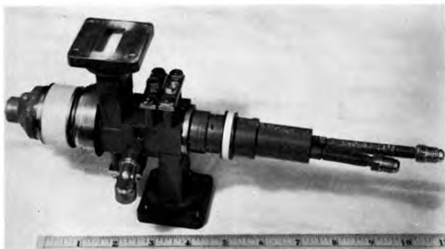
Figure 14.3(e). Type VA 806 X-band Klystron; power output 2KW (CW). (Courtesy Varian Associates.)
