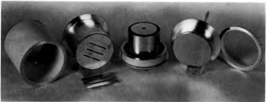
Figure 14.3(c). Components of EG&G Type 1802; from left to right: alumina ceramic cylinder 3 in. dia. \times 3\frac{1}{4} in. high; copper grid cup and grid baffle (in front); cathode assembly; copper anode cup with molybdenum face; ceramic backing ring. After Goldberg. 46 (Courtesy Edgerton, Germeshausen & Grier, Inc.)
