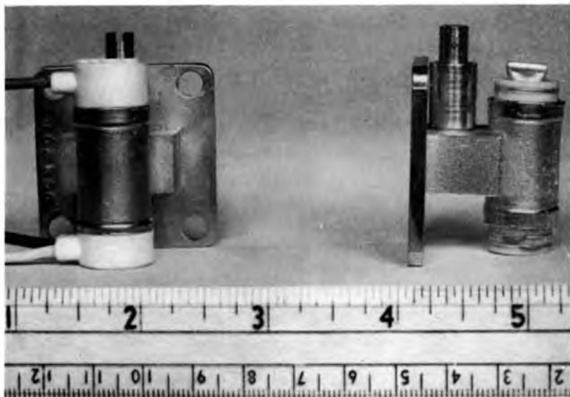
Figure 14.3(d). Type 1K20 Reflex Klystron available for X-band and K-band operation; with encapsulation (left) and without (right). Power output 75 mw; a fixed-tuned inner cavity is closely coupled to a secondary cavity outside the vacuum through a ceramic window. Tuning over a minimum range of 700MC is accomplished by a capacitive slug which is visible in the picture at the right. (Courtesy Eitel McCullough, Inc.)
