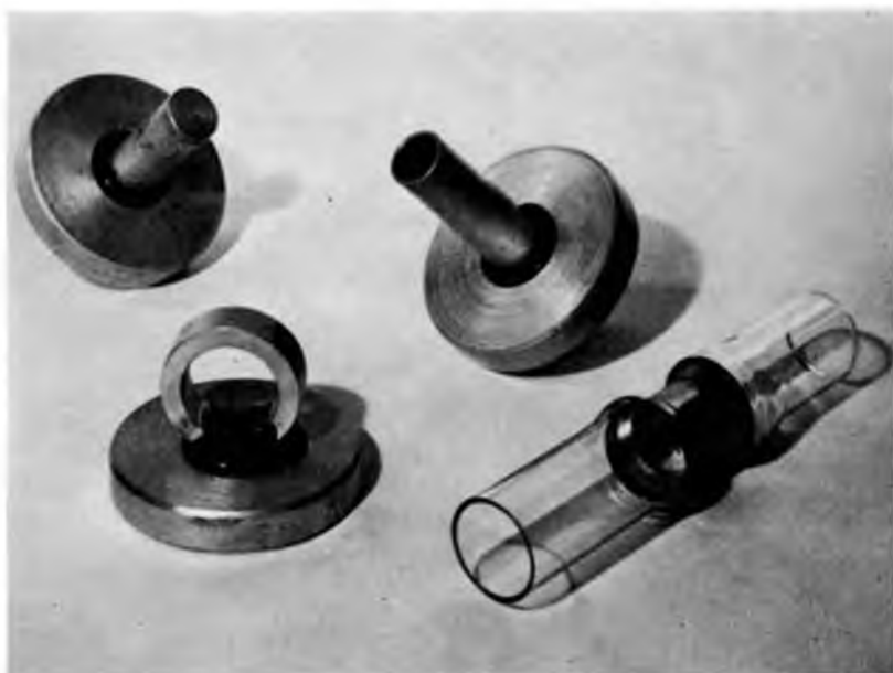
Figure 13.12(a). Three seals to bulk copper made with CSG3 glass confronted with a conventional feather edge seal (M 1765) at lower right. (Courtesy The General Electric Company, Ltd., Wembley.)
