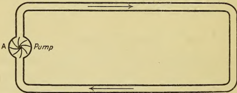
Fig. 2—Water analogy of simple electrical circuit.
