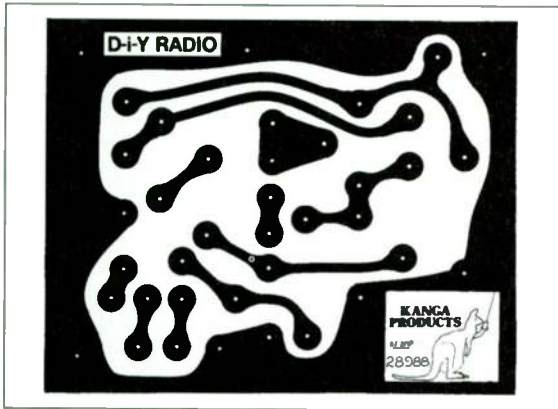
Fig 3.21. The foil pattern of the PCB – track side
