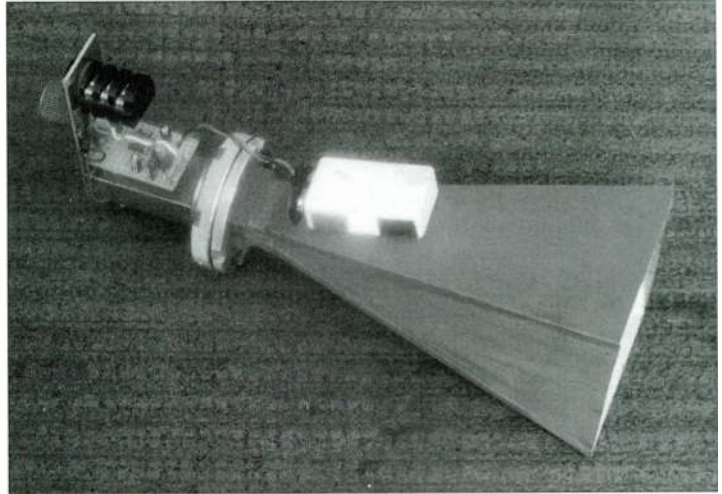
Fig 3.32. The 10GHz receiver showing the LM386 amplifier
