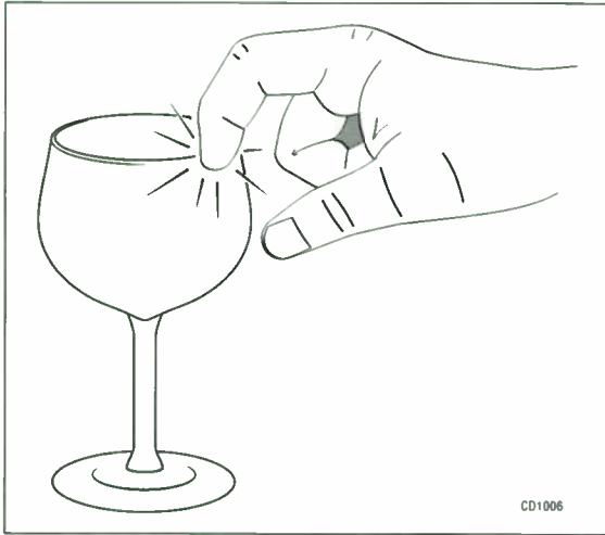
Fig 1.17. A wine glass 'rings' at a constant frequency
