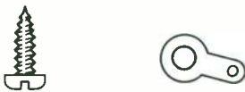
(e) Some screws do not need nuts, these are screwed into a hole which is a little too small
