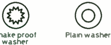
(d) Sometimes nuts work loose due to vibration, a shake proof washer under the nut will stop this
