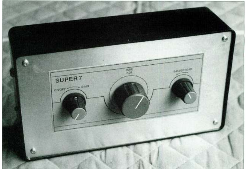
Fig 7.1. The Super 7 receiver
