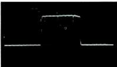
Fig. 5-12. Detected video-sweep signal waveform.
