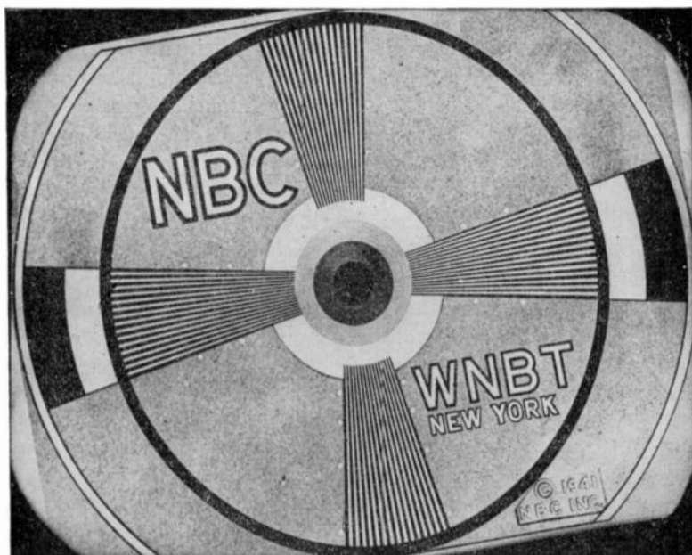
FIG. 9.16B. Incorrectly positioned image due to improper placement of deflecting coil yoke.
