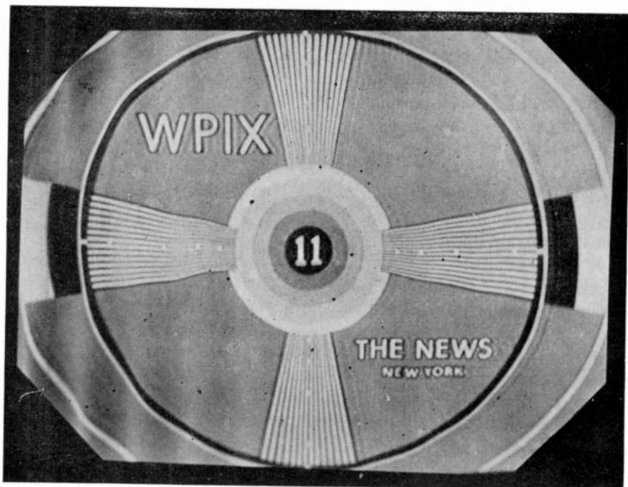
Fig. 16.18. Ripples caused by an open or wrong value of capacitor across the top half of the horizontal winding of the yoke.
