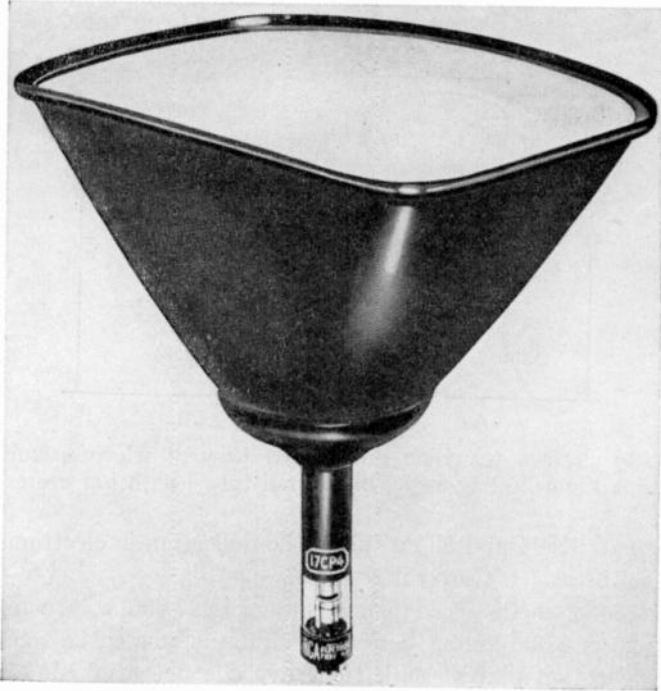
FIG. 9.32. A metal-cone picture tube.
