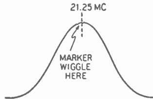
FIG. 15.16. The shape of the response curve and the position of the marker frequency when aligning the F-M, I.F. stages.
