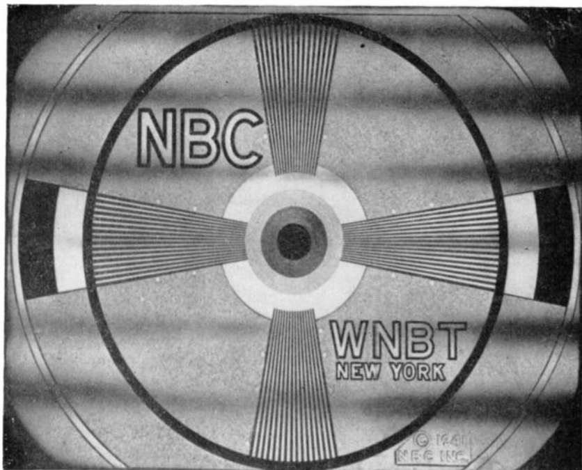
FIG. 7.24. The visual result when sound voltages reach the cathode-ray tube.
