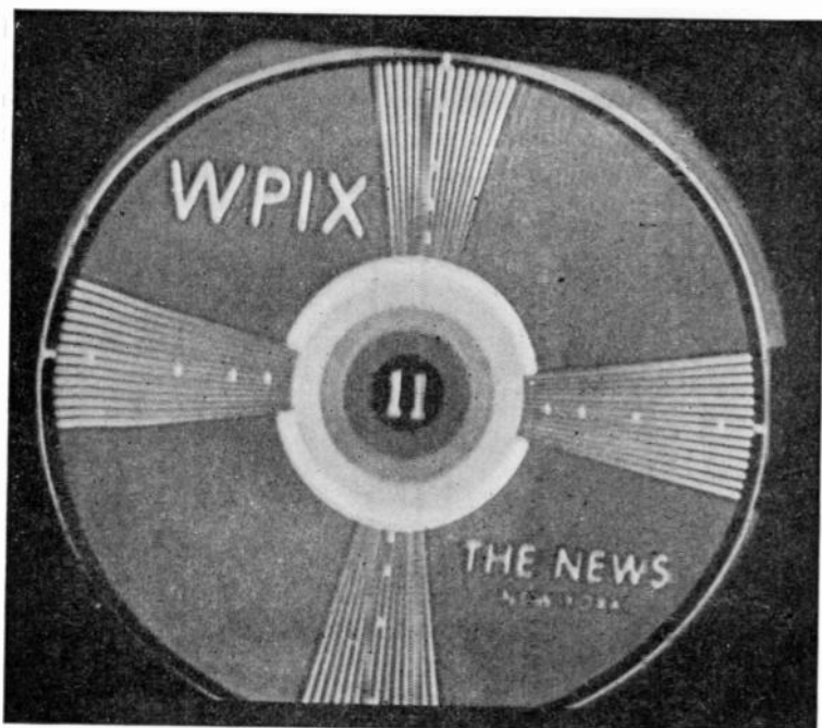
FIG. 16.16. The shadow around the outer edge of the pattern is caused by a deflection yoke which is not as close to the cone of the tube as it will go.
