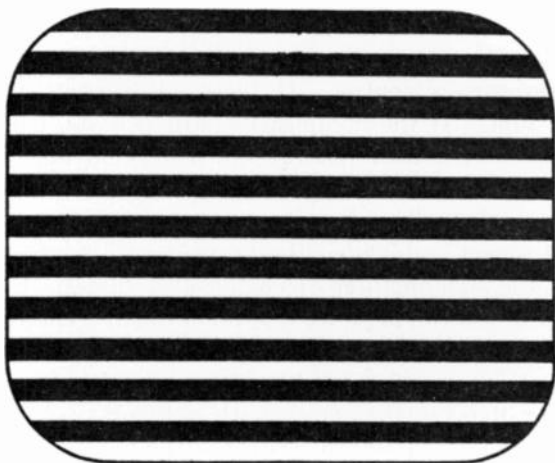
Fig. 16.28. Black and white horizontal bars for checking vertical linearity.
