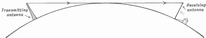
FIG. 2.6. Increasing the line-of-sight distance from the receiving antenna to the transmitter by raising both structures as high as possible.
