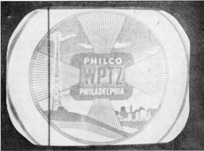
FIG. 16.35. The visual effect of a Barkhausen oscillation.
