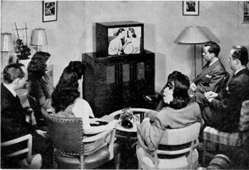
FIG. 9.36B. A projection television receiver. The image from a small projection-type tube is enlarged to permit comfortable viewing by many people.
