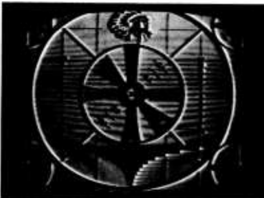
Fig. 3-22. Example of reversed-polarity smear.
