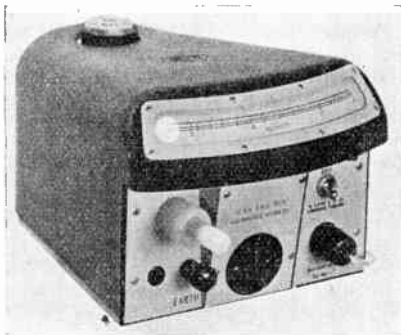
FIG. 14.—SCALAMP ELECTROSTATIC VOLTMETER.
