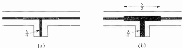
FIG. 33.—CO-AXIAL FEEDERS. Inner conductor supported by quarter-wave stubs.
