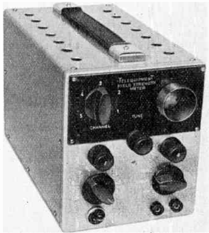
FIG. 15.—TELEVISION FIELD STRENGTH METER.
