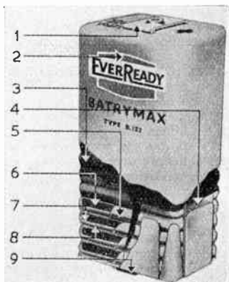
FIG. 3.—HIGH-TENSION BATTERY (LAYER-TYPE CONSTRUCTION).
