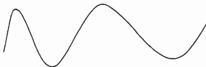
FIG. 40.—DISTORTION OF WAVEFORM OWING TO NON-LINEAR TIME-BASE.
