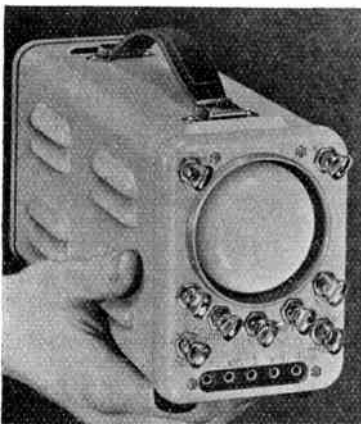
FIG. 7.—MODEL 1039M PORTABLE OSCILLOGRAPH.
