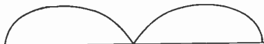
FIG. 1.—VERTICAL RESPONSE PATTERN OF A SHORT VERTICAL AERIAL, LOWER END NEAR EARTH.
