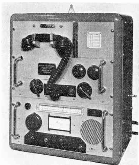
FIG. 17.—THE GR60A MARINE RADIO TELEPHONE.
