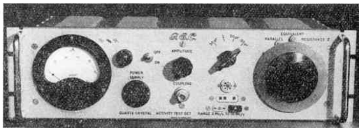
FIG. 23.—QUARTZ CRYSTAL ACTIVITY TEST SET FOR DIRECT MEASUREMENT OF THE EQUIVALENT PARALLEL RESISTANCE.
