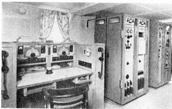
FIG. 15.—A G67 TRANSMITTER AND TWO R50M RECEIVERS FITTED IN THE RADIO CABIN OF THE Abraham Larcen WHALING FACTORY SHIP FOR LONG-RANGE COMMUNICATIONS IN THE ANTARCTIC.
