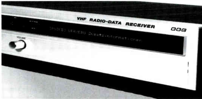
Figure 1.1 One of the first RDS demonstration receivers designed by the BBC in 1982. (Source: BBC.)
