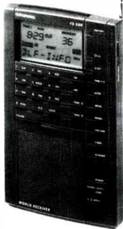
Figure 12.5 Grundig made the world's first portable RDS radio: the 1994 model YB 500. (Source: Grundig.)
