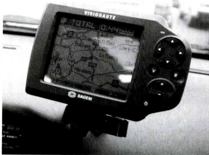
Figure 7.15 The Sagem/Médiamobile Visionaute is designed for a pay-service in Paris using the ALERT-Plus with the ALERT-C protocol. (Source: EBU.)
