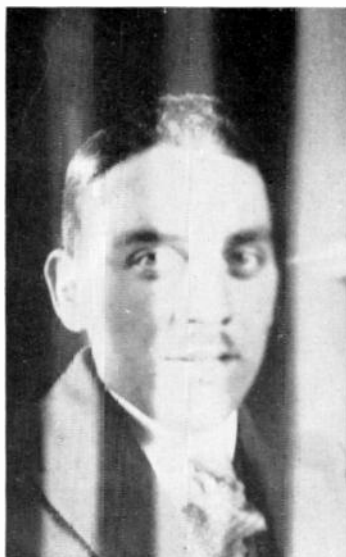
FIG. 152.—L.F. instability produces dark lines passing across the picture as represented in this illustration.
