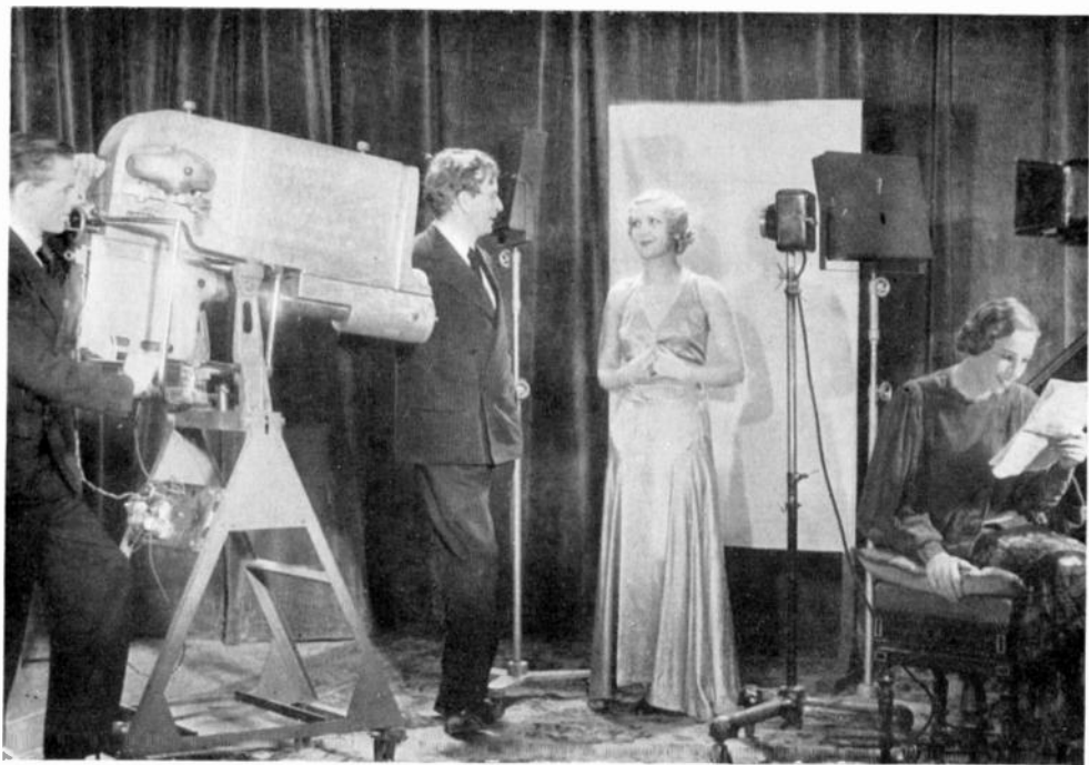
FIG. 128. — A photograph of an actual television transmission being carried out. On the left may be seen a portable transmitter.
