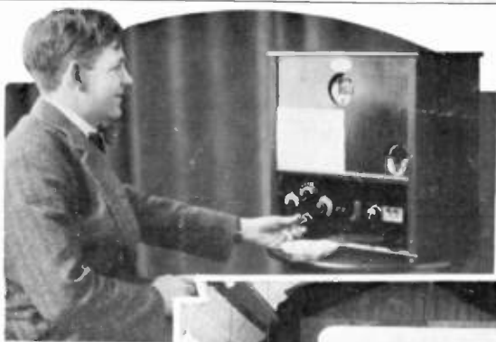
FIG. 158 (left).— One of the first experimental "all-in" television receivers. FIG. 159 (below). A small cinematype screen upon which television images have been projected
