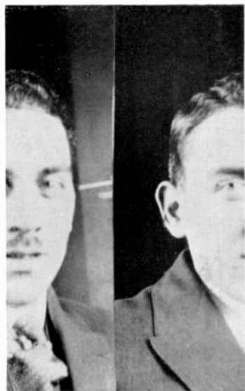
FIG. 155.—Another fault which occurs, due to the lack of synchronism.
