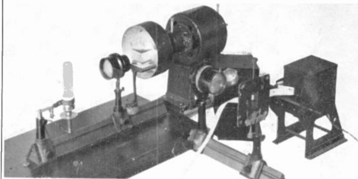
FIG. 21.—A complete transmitting equipment using an apertured drum.
