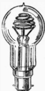
FIG. 223.—The "bee-hive" lamp so called because of the shape of the electrode.
