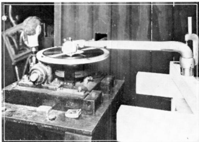
FIG. 87.—A dummy's head acting as a subject for making a test phonovision record, this latter process being visible in the foreground.
