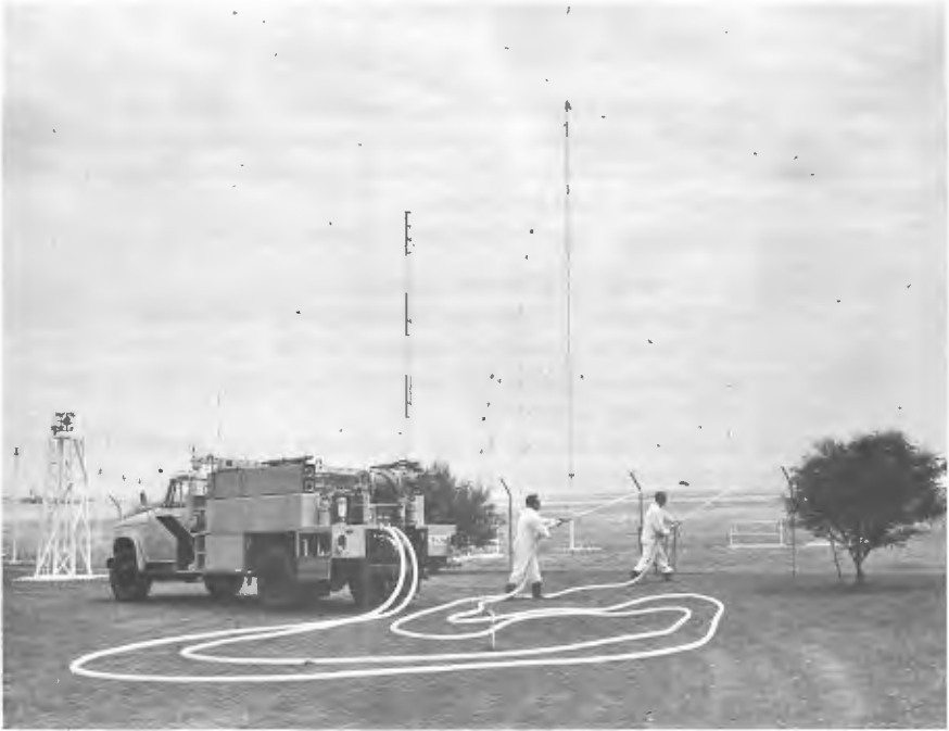
Figure 32.2 Typical fire fighting unit for dealing with station grass fires
