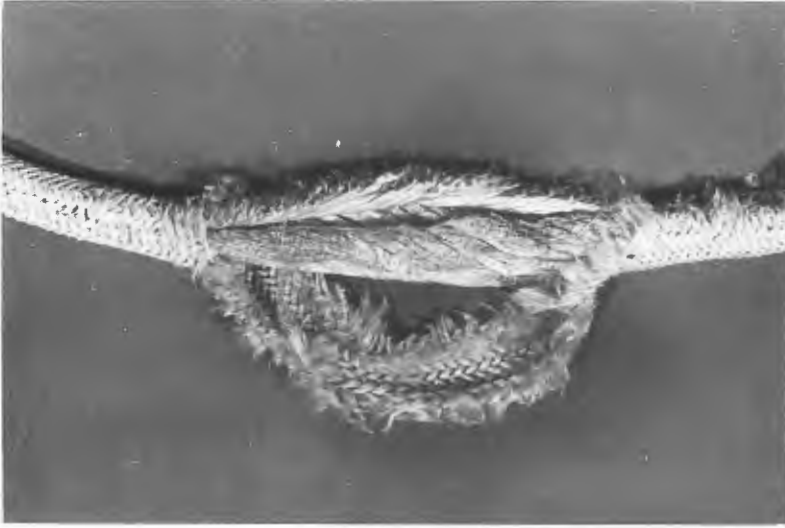
Figure 41.8 Deterioration of polypropylene rope
