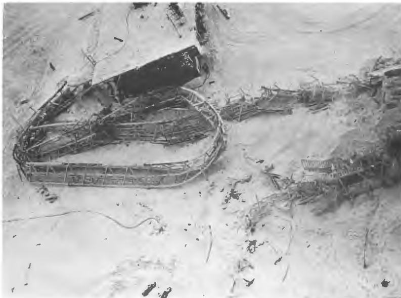
Figure 26.17 Mast wreckage near transmitter building (Courtesy Finnish Broadcasting Co. Ltd)
