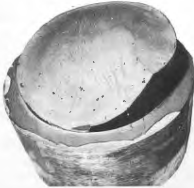
Figure 26.14 Bottom section of fractured insulator
