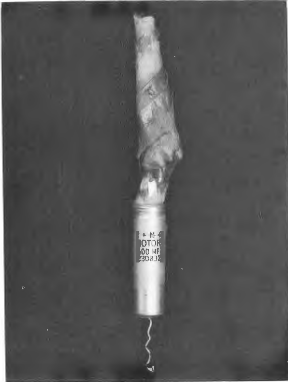
Figure 20.1 Exploded electrolytic capacitor
