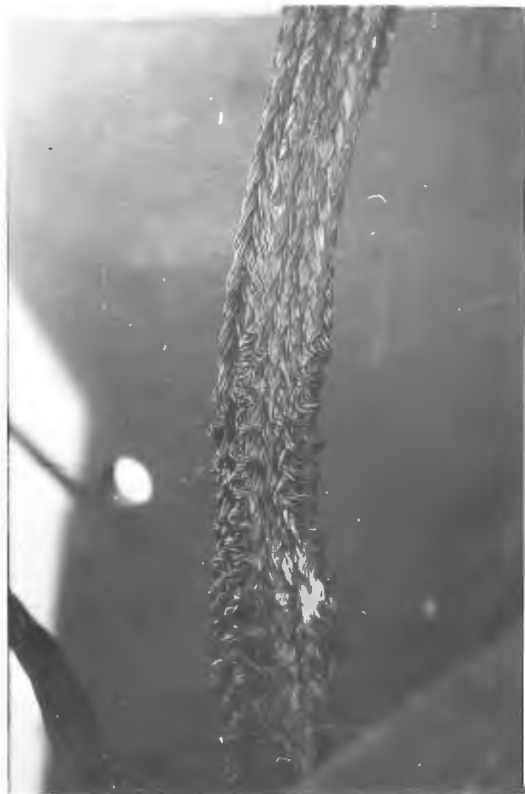
Figure 38.12 Displacement of braid wires following lightning stroke
