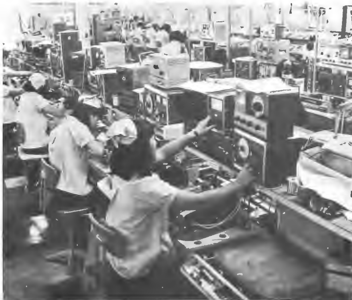
Figure 48.1 Production line testing of amplifiers (Courtesy JETCO)
