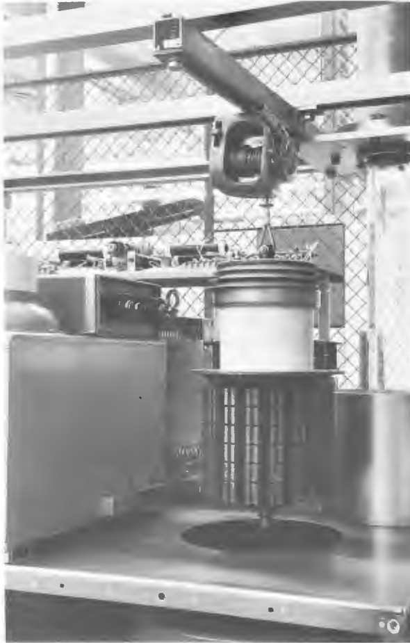
Figure 23.4 Rockwell-Collins Tubelifting Device (Courtesy Rockwell International)
