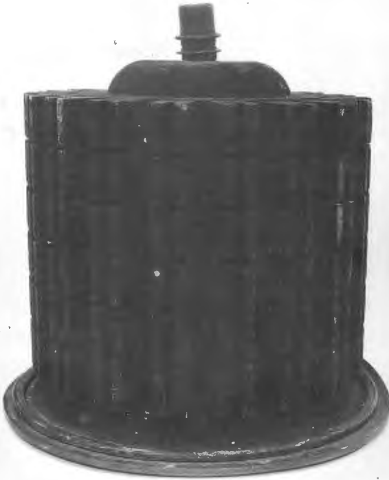
Figure 42.4 Scale on plate of vapour phase cooled power tube
