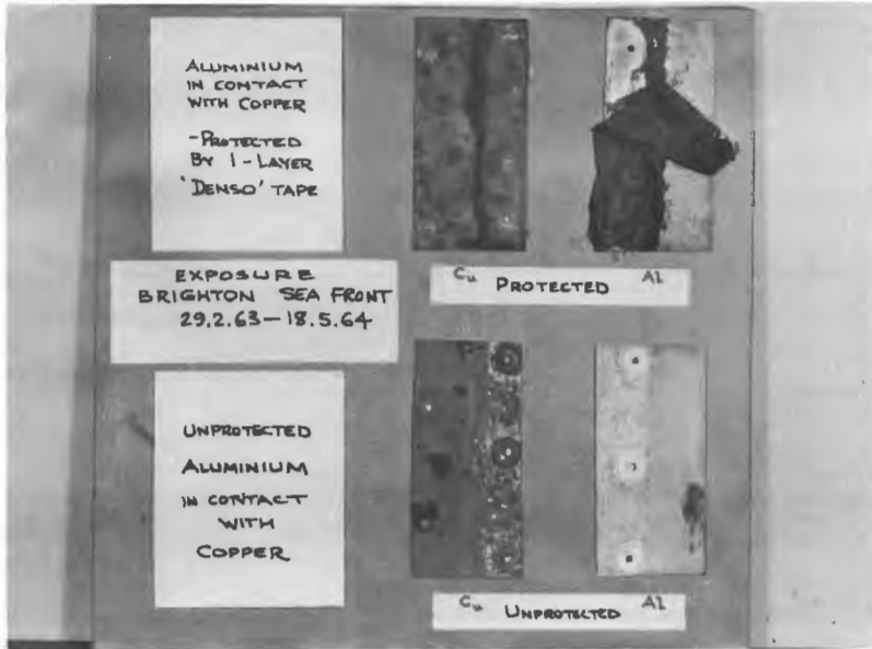
Figure 42.8 Tests with copper-aluminium contact
