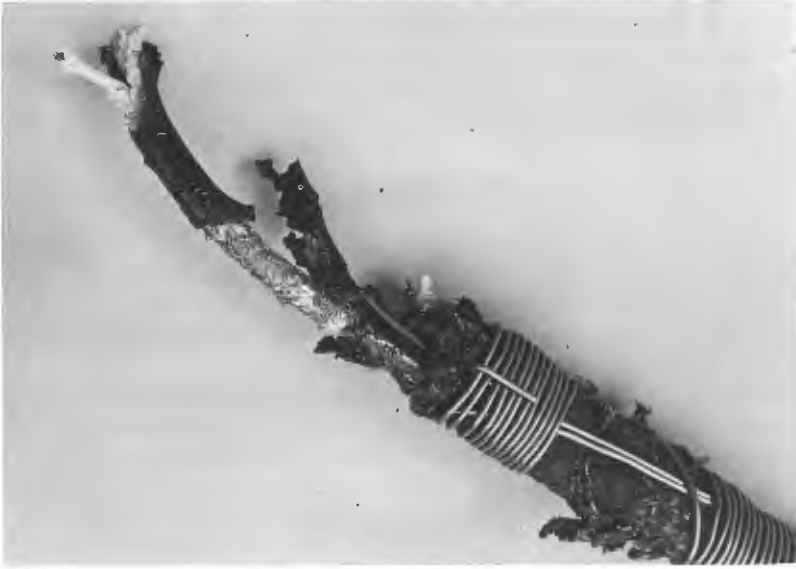
Figure 40.11 Antenna feeder damaged by parrots
