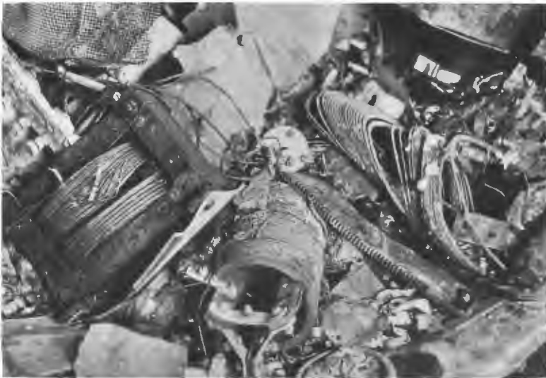
Figure 34.5 Destruction of combustible materials in transmitter fire
