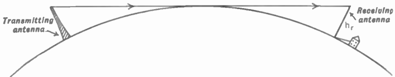
FIG. 4.7. Increasing the line-of-sight distance from the receiving antenna to the transmitter by raising both structures as high as possible.
