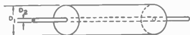
FIG. 5.9. A coaxial cable. D_1 is the inside diameter of the outer conductor; D_2 is the outside diameter of the inside conductor.
