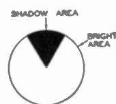
FIG. 9.35C. The eye opening when the grid becomes more positive.
