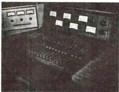
Fig. 5. Horizontal Control Panel with Slide-type Mixing Pots.
