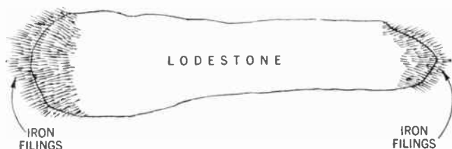
Figure 30-4. Iron filings attracted to the poles of a magnet.
