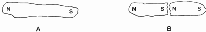
Figure 30-7. A—Poles on a magnet. B—Arrangement of poles on a magnet broken in half. Note that each piece has two poles.
