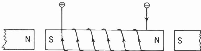
Figure 30-22. The electromagnet, having rotated a half turn, now comes to rest with unlike poles facing each other.
