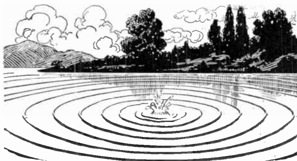
Figure 2-1. Ripples caused by throwing a stone into a still pond. These ripples travel in ever-widening circles from the point of disturbance.
