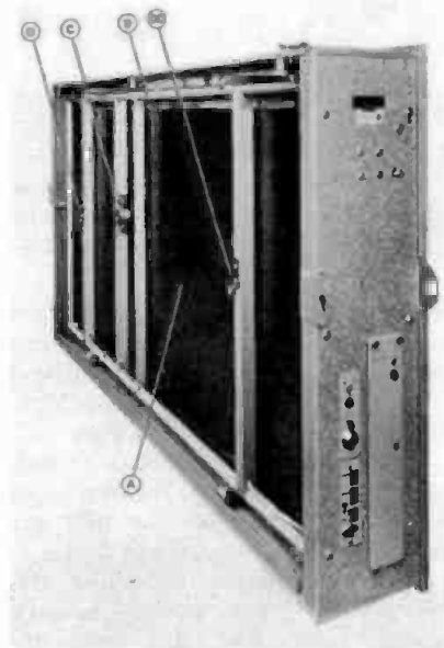
Fig. 2-130B. Rear view of EMT Model 140st stereophonic reverberation unit showing the two pickup units at the ends and the drive unit in the center. (Courtesy, Gotham Audio Corp.)
