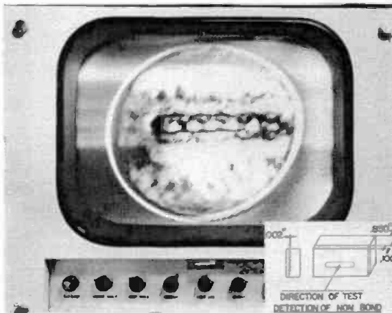
Fig. 25-215C. Ultra-Scan picture of a nonbond. Frequency, 2 MHz. Material, aluminum. The nonbond area is indicated by the dark pattern in the center of the display.
