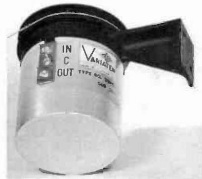
Fig. 13-111A. A diameter equalizer-attenuator control manufactured by Cinema Engineering Co. The cord is attached to the cutting-head carriage.
