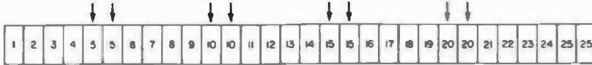
Fig. 2-131D. Playback with an expansion of 20 percent. Every 5th section is repeated as indicated by the arrows.
