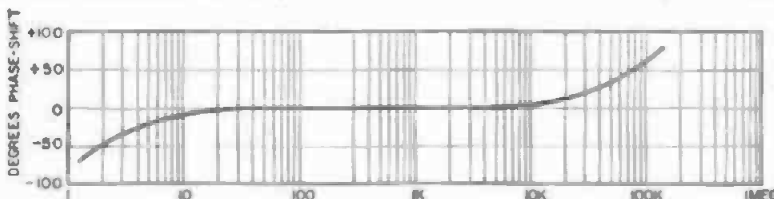
Fig. 12-232E. Phase shift of the power amplifier in Fig. 12-232A.
