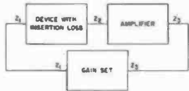
Fig. 23-55B. Measuring high insertion loss using a gain set.
