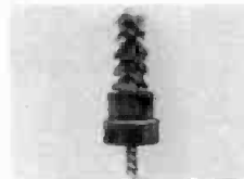
Fig. 24-13. Western Electric bristle brush for polishing the interior surfaces of a jack sleeve.
