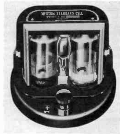
Fig. 23-195B. Weston Standard voltage cell, unsaturated cadmium type.
