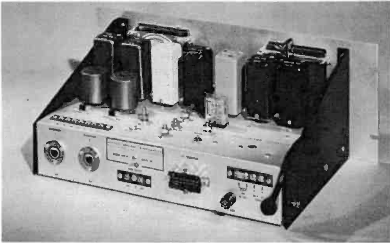
Fig. 17-180B. Stancil-Hoffman Model ARP70 transistor amplifier system for mixing, recording, or reproducing either magnetic tape or film.
