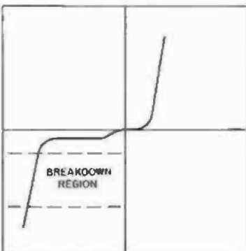
Fig. 11-148A. Zener forward and reverse current characteristics.
