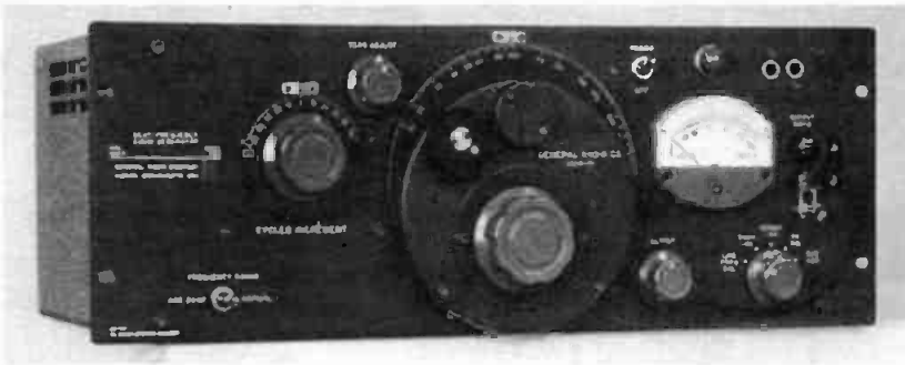
Fig. 22-51C. General Radio Co., Model 1304B beat-frequency oscillator.
