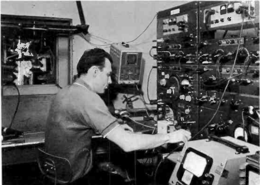
Fig. 2-83D. Routine production test equipment outside the Altec-Lansing anechoic chamber. The device to be tested is hung from a pulley-and-cord arrangement for ease of operation and orientation.
