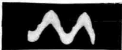
Fig. 23-125F. Waveform at output of unstable negative-feedback amplifier with an 0.01- \mu\text{F} capacitor connected across a 16-ohm resistive termination. Waveform is an intermodulation signal of 40 and 2000 Hz. The wide white band is high-frequency oscillation superimposed on the low-frequency signal.
