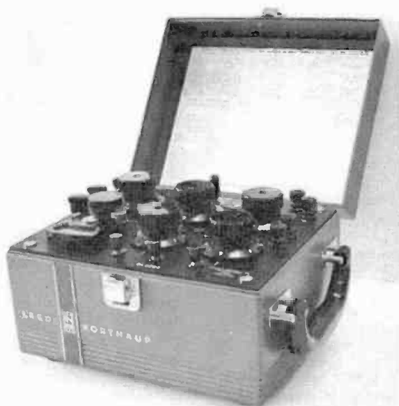
Fig. 22-21. The Leeds and Northrup Model 5430-AM Wheatstone bridge.
