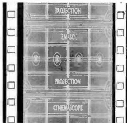
Fig. 19-129. Test chart for adjusting wide-screen projection images, using an anamorphic lens system.
