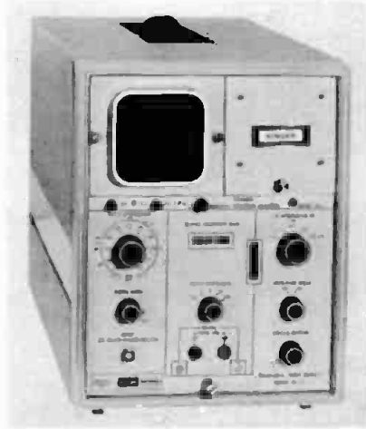
Fig. 22-93A. Singer Co., Metrics Div., Model TA-2 universal spectrum analyzer, with AL-2 plug-in module for 20 Hz to 35 kHz spectrum analysis.
