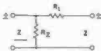
(d) Between impedances of equal value, in the direction of the shunt arm.
