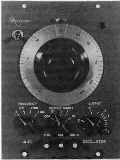
Fig. 22-49A. Front panel view of Waveforms Inc. Model 401B audio oscillator.
