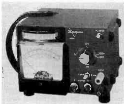
Fig. 22-140C. Logarithmic ac volt and frequency meter Model 620A manufactured by Waveforms Inc. An external frequency source is required with this instrument.
