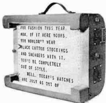
Fig. 2-72A. Teleprompter unit with script. The "hot line" appears to the right of the plastic pointer.
