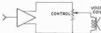
Fig. 20-141. Proper connections for a potentiometer or L-type attenuator in a loudspeaker transmission line.
