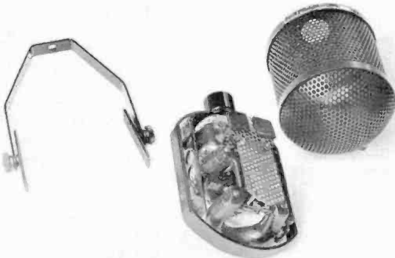
Fig. 4-60A. Interior view of an early (1935) Western Electric RA-1142A unidirectional microphone for motion-picture sound recording. Now obsolete, but it is still of historical interest.
