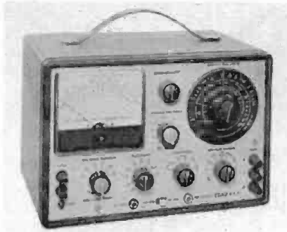
Fig. 22-34B. EICO Electronic Instrument Co., Inc. Model 965 FaradOhm bridge analyzer.
