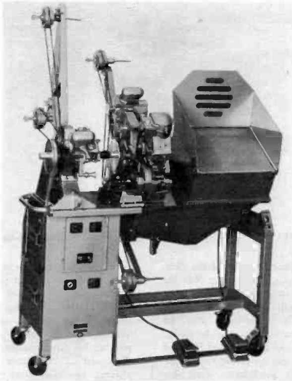
Fig. 18-198C. Magnasync-Moviola combination 16/35-mm preview-type editing machine.
