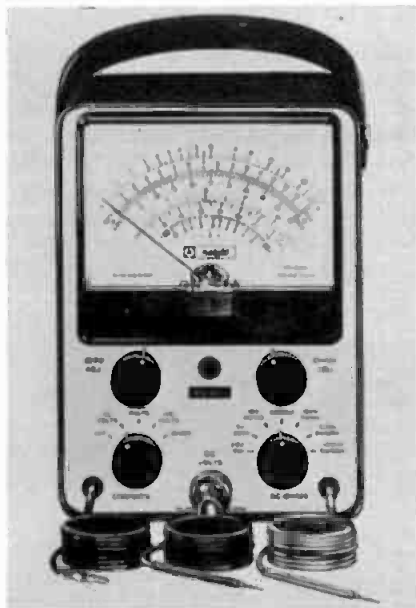
Fig. 22-11B, Allied Radio Corp. Model KG 620 vacuum-tube volt-ohmmeter.
