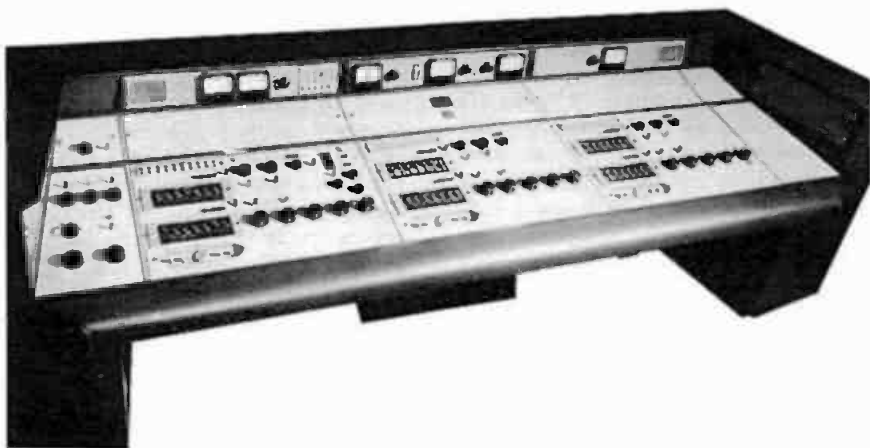
Fig. 9-46A. Three-section rerecording (dubbing) console, designed by H. M. Tremaine and constructed by McCurdy Radio Industries, Canada.
