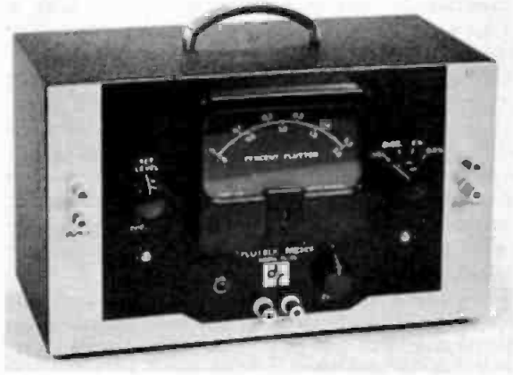
Fig. 22-41A. Sentinel Inc. Model FL-3D-1 flutter and wow meter.
