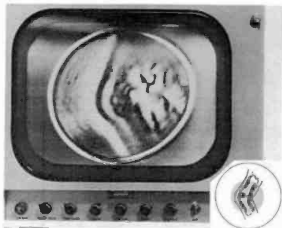
Fig. 25-215D. Ultra-Scan display of a biological examination. Frequency, 2 MHz. Material is bone, blood, and tissue.
