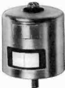
Fig. 17-147A. A 16-mm magnetic recording head.
