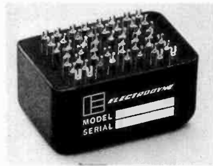
Fig. 5-99A. Electrodyne Model ACN-1 active combining network.
