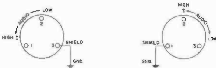
Fig. 4-95. Pin count used on microphone cables.
