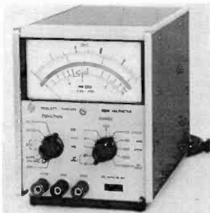
Fig. 22-11D. Transistor multipurpose meter, Model 427A manufactured by Hewlett-Packard.
