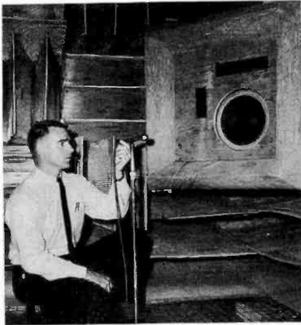
Fig. 2-83B. Testing a microphone in the Electro-Voice anechoic chamber.
