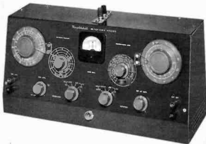
Fig. 22-33B. Heathkit Model IB-2A impedance bridge.
