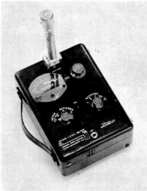
Fig. 22-94A. General Radio Co. Model 1551C sound-level meter.
