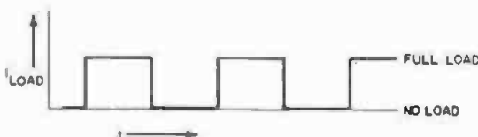
Fig. 21-115B. Square wave applied across the output terminals to measure the recovery time.
