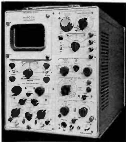
Fig. 22-70A. Marconi Instruments Ltd. (England) Model TF-2200 cathode-ray oscilloscope designed for plug-in preamplifier operation. The preamplifier is plugged-in at the lower left. (Courtesy, Canadian Marconi Instruments Ltd.)
