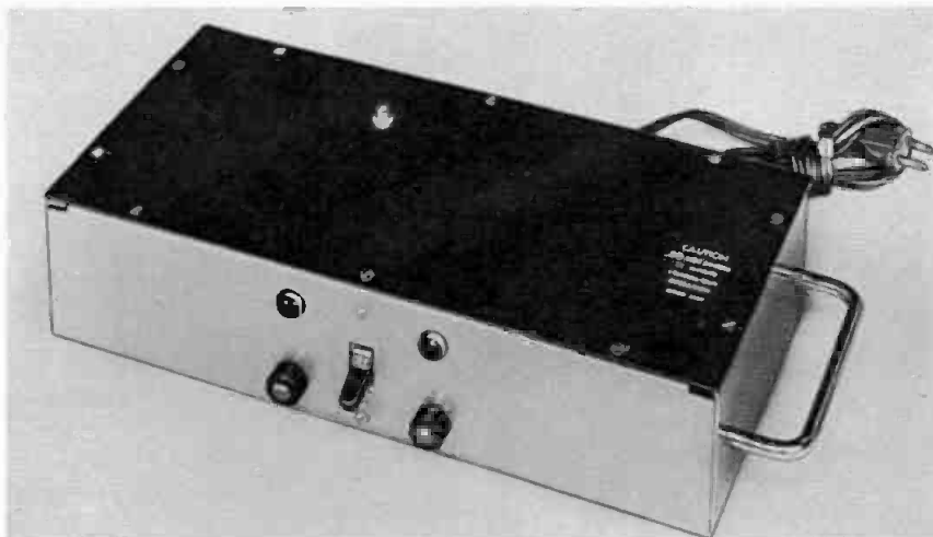
Fig. 17-65A. A magnetic tape or film bulk eraser manufactured by the Hollen Corp.
