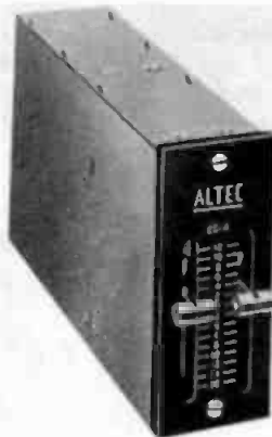
Fig. 6-100A. Altec-Lansing microphone equalizer Model 9060A.
