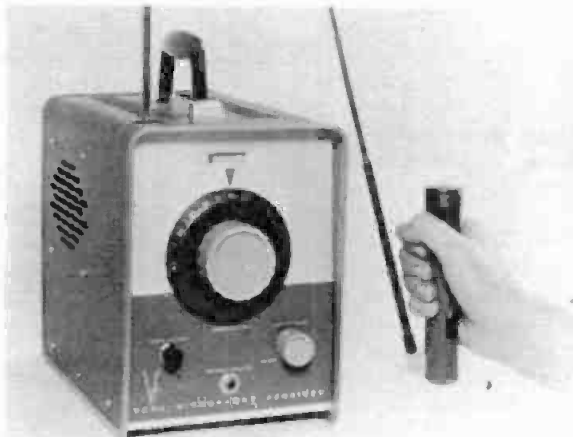
Fig. 4-72A. Vega Electronics Corp. wireless microphone system. The microphone and its fm radio transmitter are shown at the right, and the receiver at the left.
