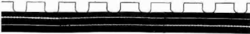
Fig. 18-255. A typical push-pull crossover test for a push-pull variable-area photographic film recorder (print).
