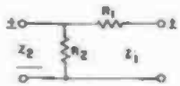
(c) Impedances unequal, and impedance match is toward the smaller of the two.
