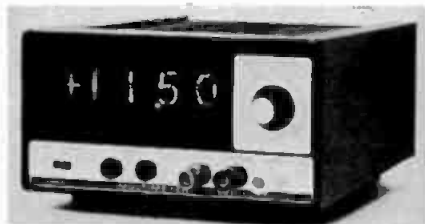
Fig. 22-143A. Front panel view of Fairchild Instrumentation Model 7050 solid-state digital multimeter, using dual-slope integration techniques with 0.1-percent accuracy.
