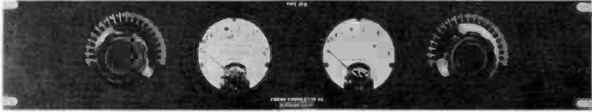
Fig. 10-22. An early type dual volume indicator panel manufactured in 1939 and now obsolete. (Courtesy, Cinema Engineering Co.)
