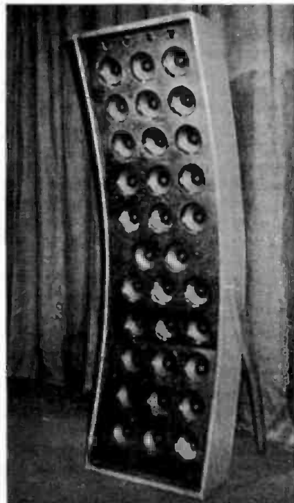
Fig. 20-184A. Series-parallel array using 32-individual speaker units. (Courtesy, H. F. Sales, Vancouver B.C., Canada)
