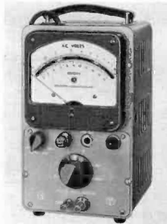
Fig. 22-102A. Ballantine Laboratories Model 300G logarithmic vacuum-tube voltmeter.
