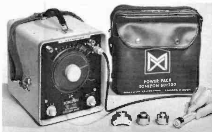
Fig. 25-216A. Model-SO-300 ultrasonic thickness-measuring gauge manufactured by Magnaflux Corp.
