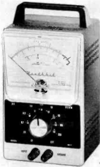
Fig. 22-99A. Heathkit Model IM-21 audio-frequency vacuum-tube voltmeter.
