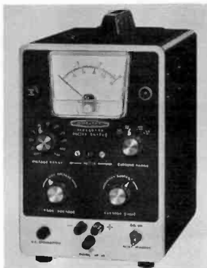
Fig. 21-128A. Heathkit Model IP-20 regulated power supply (solid-state).
