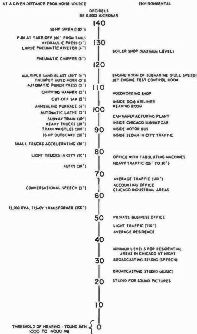
Fig. 1-117A. Typical overall sound levels encountered in daily life. The levels are in reference to 0.0002 microbar. (Courtesy, General Radio Co.)
