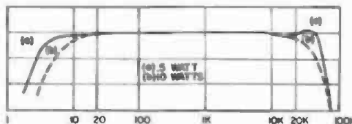
Fig. 12-131. Frequency response of a wide range high-quality audio amplifier at 0.5 and 10 watts output.
