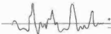
Fig. 1-64B. A typical speech oscillogram showing the energy or amplitude of the positive and negative peaks which are not symmetrical.
