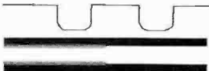
Fig. 18-100. Attack-time test for compressor amplifier, opening time 3 milliseconds.
