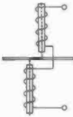
Fig. 17-37A. Longitudinal method of magnetization.
