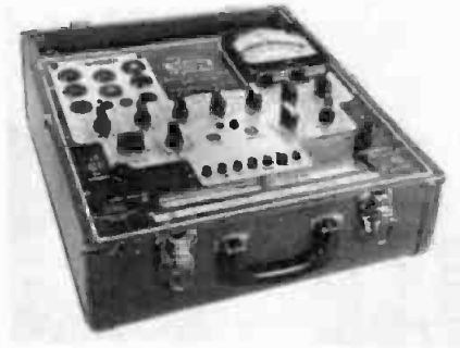
Fig. 22-115A. Dynamic mutual conductance tube tester Model 9-66A manufactured by Stark Electronic Instruments (Canada).
