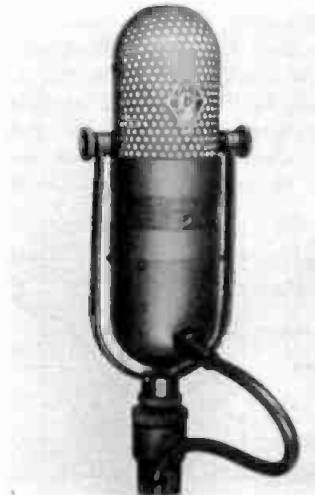
Fig. 4-77A. RCA Model 77DXMI-4045-F polydirectional microphone.
