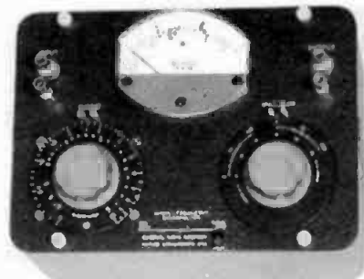
Fig. 22-43A. General Radio Co., Model 546-C audio frequency microvolter.
