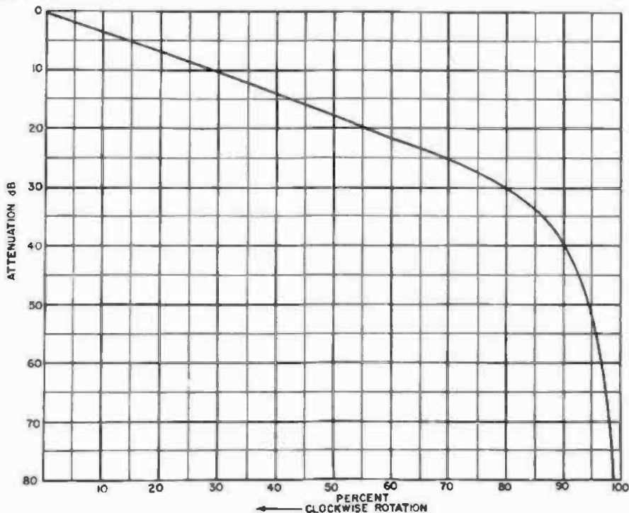
Fig. 5-81. Attenuation versus percent rotation for a typical mixer control.
