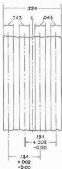
Fig. 17-150C. Sound track dimensions for four-track, \frac{1}{4} -inch tape, monophonic or stereophonic recording.
