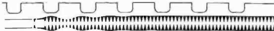
Fig. 18-65B. A maladjusted noise-reduction shutter opening test, showing shutter bump at the start of the opening (negative).
