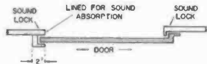
Fig. 2-69. Plan view of a typical sound-stage door installation. The sound lock on the left side starts at the floor and continues to the top and across to the right side. Rollers at the bottom support the weight of the door when it is opened.
