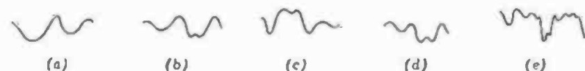
Fig. 23-125D. Intermodulation products of a McIntosh MC-30 amplifier with 16-ohm resistive load termination. The connection of a capacitor across the load termination makes no change in the distortion components. (a) 10 watts output, IM = 0.14%. (b) 20 watts output, IM = 0.20%. (c) 25 watts output, IM = 0.20%. (d) IM = 0.21%. (e) IM = 0.25%.
