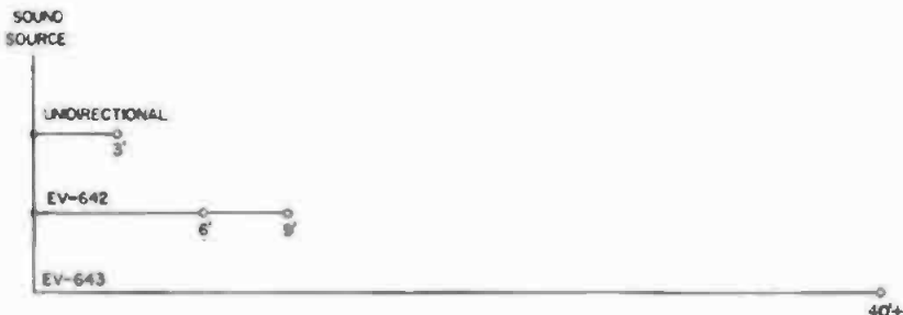
Fig. 4-102. Comparison of standard unidirectional microphone and Electro-Voice Models 642 Cardline, and 643 long-range pickup.
