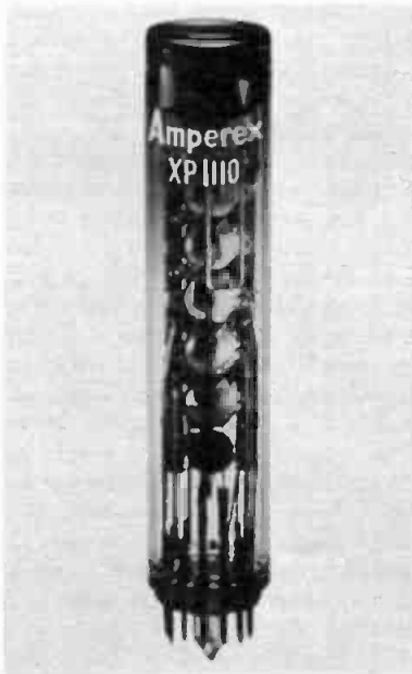
Fig. 11-32A. Amperex Electronic Corp. XP 1110 10-stage, photocathode photomultiplier tube.
