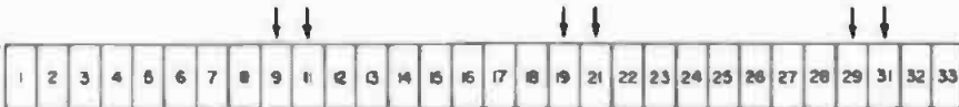
Fig. 2-131E. Playback with a compression ratio of 10 percent. Every 10th section is omitted.
