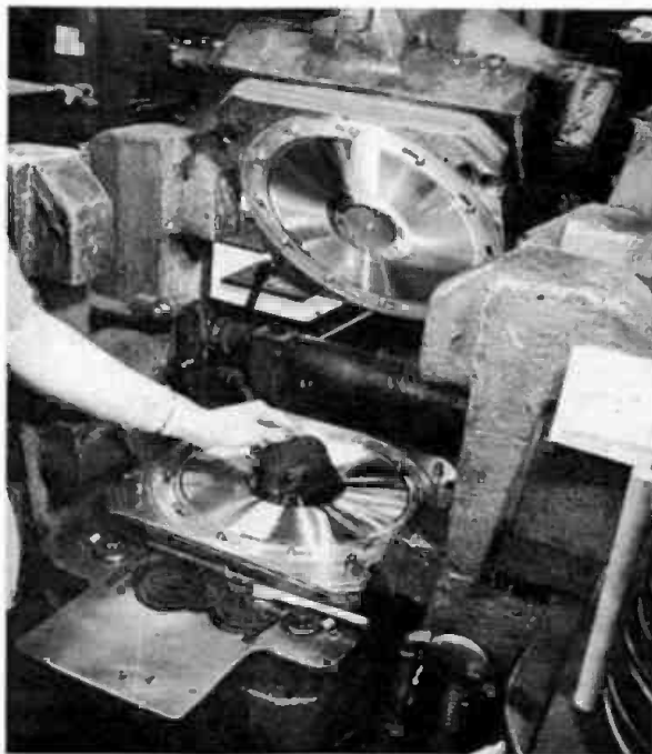
Fig. 13-127. Disc record press as used in the RCA Victor record pressing plant at Camden, N.J.
