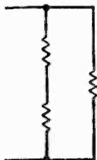
FIG. 2-23. Parallel resistance combination.
