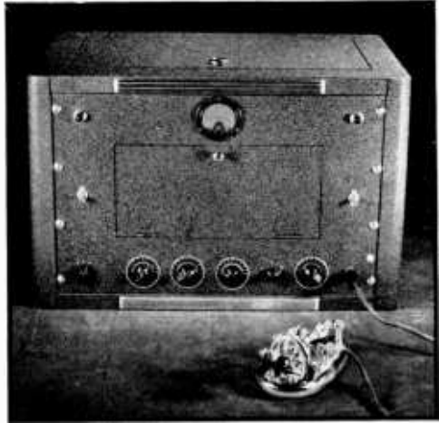
Figure 15. 150-WATT C.W. TRANSMITTER. This completely self-contained c.w. transmitter delivers 150 watts on 20, 40, or 80 meters.
