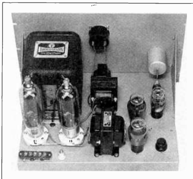
Figure 17. 203-Z SPEECH-MODULATOR FOR INPUTS TO 800 WATTS. The complete speech amplifier and class B output stage are built upon a single relay-rack panel and its associated chassis. The speech amplifier incorporates automatic peak limiting and uses a pair of 2A3's as drivers for the 203-Z's.
