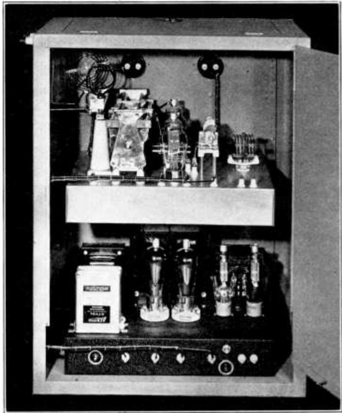
Figure 14. REAR VIEW OF R.F. AMPLIFIER AND MODULATOR.
