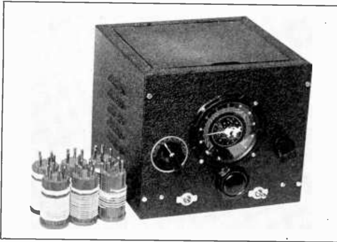
Figure 17. FRONT VIEW OF THE CONVERTER INSTALLED IN ITS METAL CABINET.
