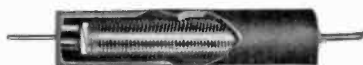
Cross Section—showing progressive interleaved windings for higher resistance values in less space.
