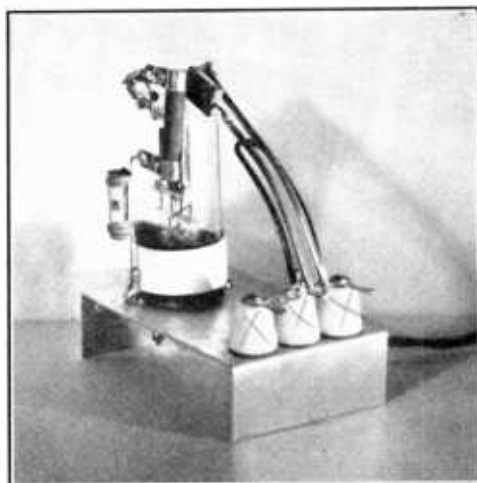
Figure 9. 8-WATT HY-75 224-MC. OSCILLATOR
