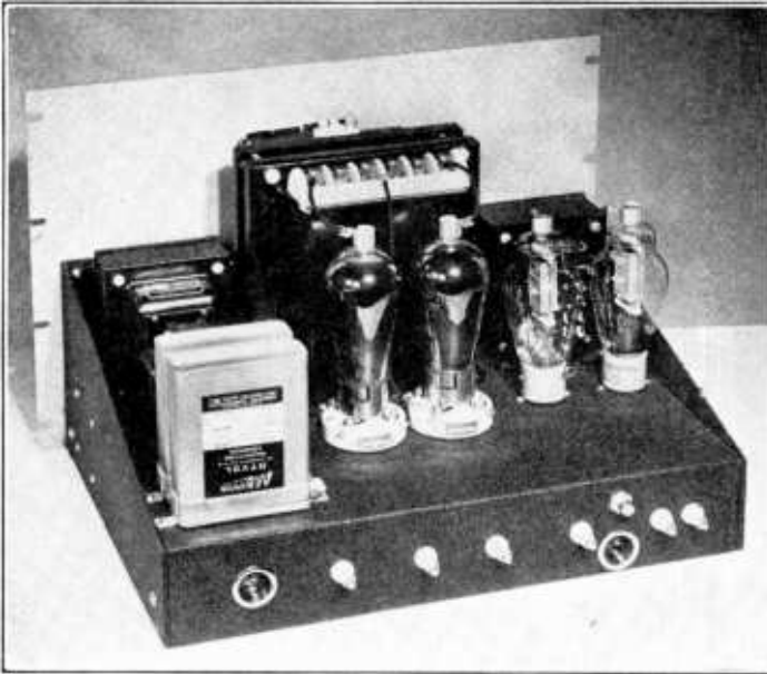
Figure 12. POWER SUPPLY AND 811 MODULATOR.
