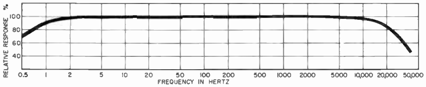
Figure 4-8. Electrical frequency response of Type 1553-A Vibration Meter, FUNCTION switch at ACCEL, power switch at 2-20,000 Hz.
