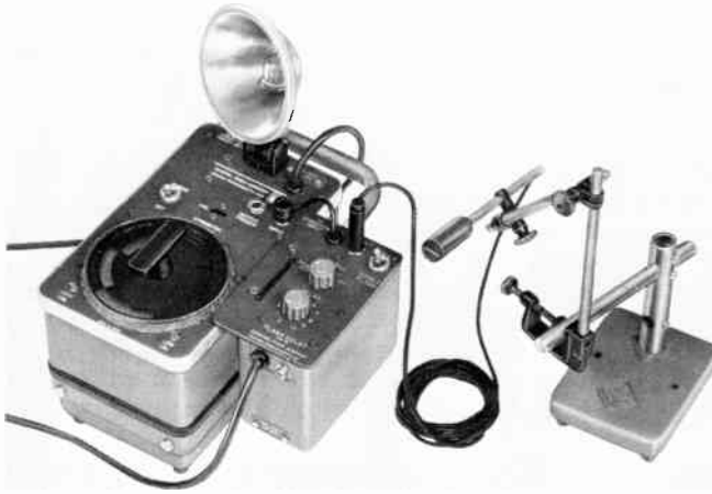
Figure 7-12. An electronic stroboscope arranged for triggering from a photoelectric pickoff with an adjustable delay. These instruments were used to obtain the photographs of the cam and follower.
