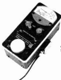
View of the calibrator with Type 1560-PS2 Vibration Pickup attached.
