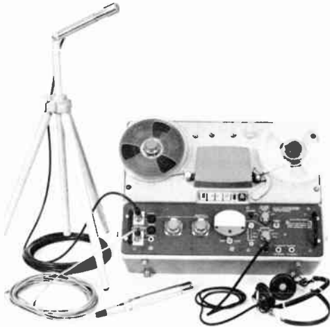
Figure 4-28. The 1525-A Data Recorder with Pre-amplifiers and microphones at both input channels and headphones at its "monitor" jack.
