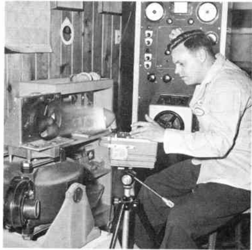
Figure 8-7. Acoustic Research, Inc. studies acoustic-radiator diaphragms with the Type 1531-A Strobotac® electronic stroboscope. A band of fine flock fiber is applied to the radiator's surface. Under stroboscopic light, nodal points and radiator break-up zones are pinpointed by the degree of fiber vibration along the band of flock. Former methods limited measurements to 1 kHz. The high intensity, short-duration flash of this new stroboscope extends these measurements to 20 kHz.
